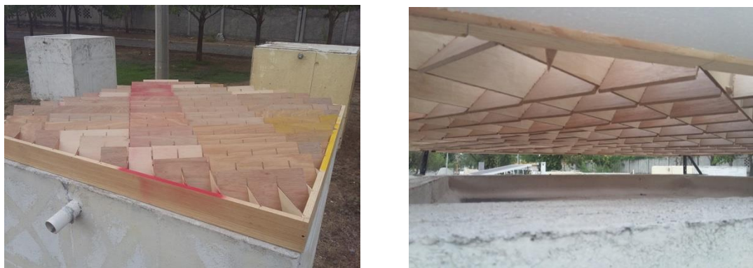
Figure 21: Pictures of the proposed roof device placed on the experimental models attached and separated from the parapet.
