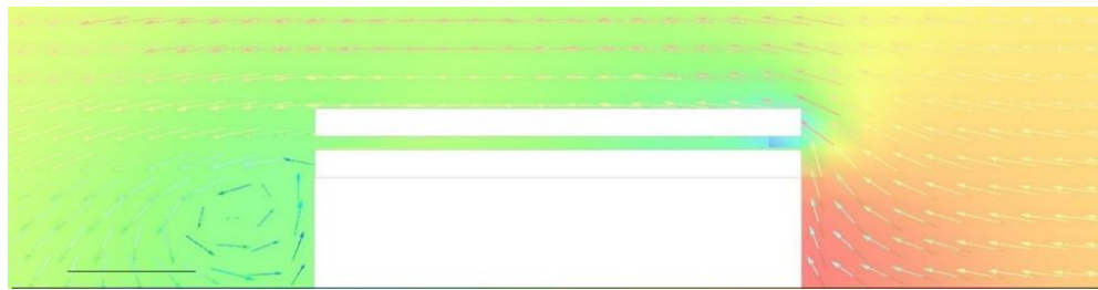
CFD analysis of the device with 0.10m cavity.
