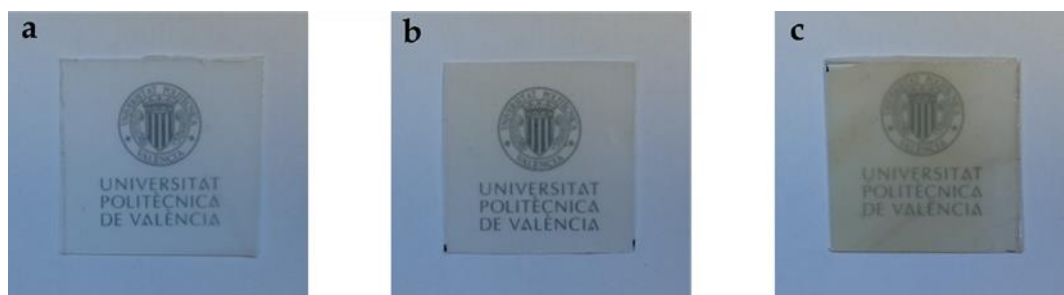
Figure 1. Visual appearance of the bio-based high-density polyethylene (bio-HDPE) films containing different amounts of gallic acid (GA): (a) Bio-HDPE; (b) Bio-HDPE + 0.3GA; (c) Bio-HDPE + 0.8GA.
