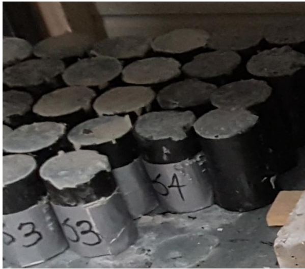
Fig. 1: Casting concrete specimens in cylindrical plastic moulds
