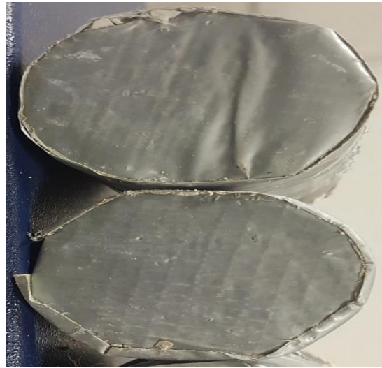
Fig. 2: Self-adhesive tape fixed at the bottom of cylindrical moulds
