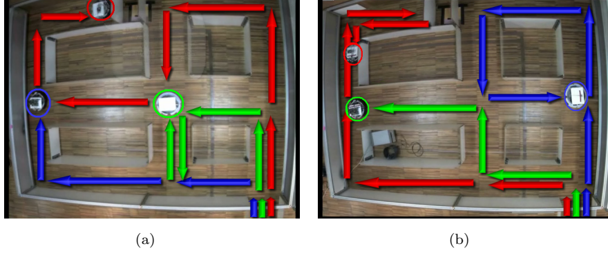
Figure 18: (a) Three robots exploring a gas free environment (b) Three robots exploring the environment and finding the odor sources.
