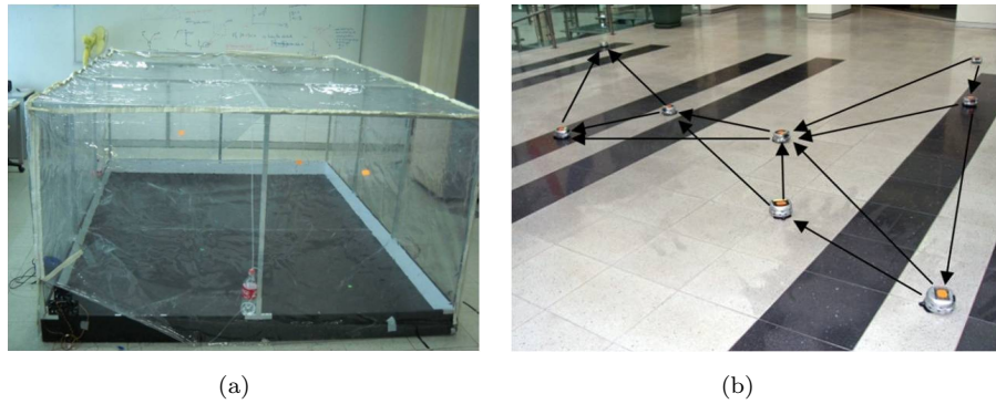
Figure 17: (a) The experimental facility, Olfactory Arena; (b) Final robot positions in RSSI based triangulation.
