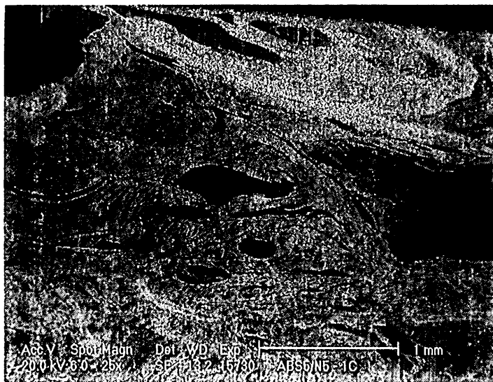
Figure 6.24: SEM Photomicrograph of ABS/Nylon 6 (50:50) Blend at 25X magnification
