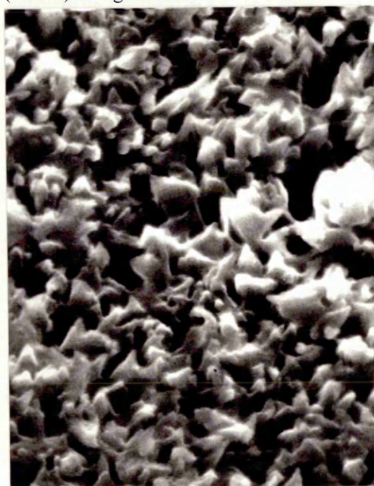
Figure 5.12 Crude FePc as deposited (XL30). Magnification 40000X.
