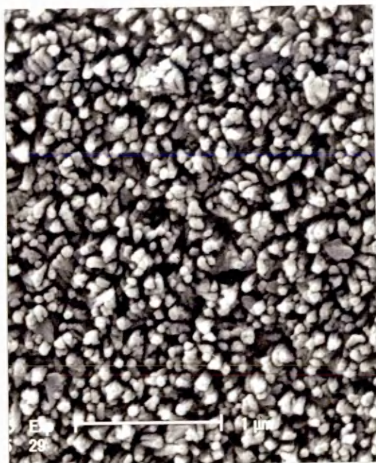
Figure 5.5 Pure FePc as deposited (XL40). Magnification 30000X.
