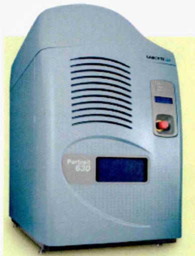
Figure 2-2: A Portrait 630 multi-reagent spotter, which uses acoustic droplet ejection technology to dispense matrix onto samples.
