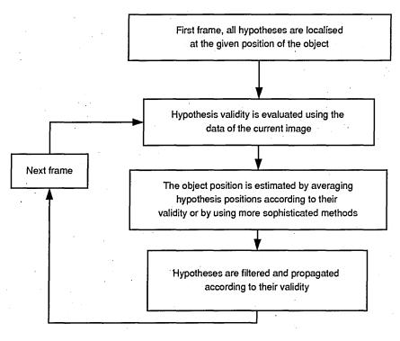
Figure 3.1: Particle filtering stages.
