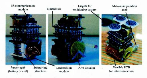
Figure 1.6: The MiCRoN robot.
