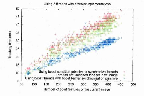
Figure 6.11: Comparison of the parallelisation on 2 processors using different implementations
