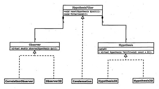
Figure 3.13: UML diagram of the first design of the particle filter
