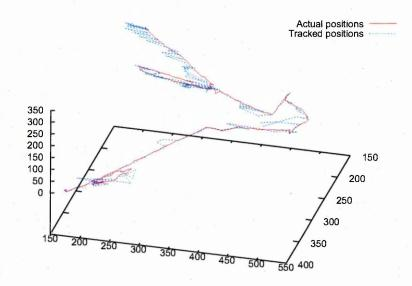
Figure 6.57: Comparison of the tracked positions and the manually determined positions of the pipette tip when using using the Canny edge detector with the second set of parameters.
