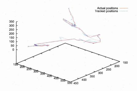
Figure 6.56: Comparison of the tracked positions and the manually determined positions of the pipette tip using the Canny edge detector with the first set of parameters.
