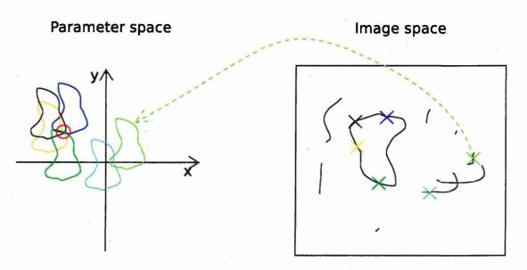
Figure 2.5: Diagram to explain the Hough transform, see text for explanation.
