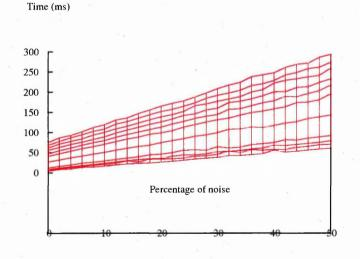
Figure 6.40: The same graph as in figure 6.39 but with a different viewpoint. This shows how the level of noise affects the tracking time
