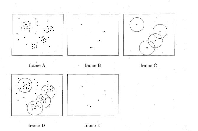
Figure 3.10: In frame A points represents particles. Frame B shows the thresholded particles. In frame C, the boundaries show how these particles are grouped and can be seen as the set bounds . Frame D shows how the other particles are collated into the corresponding sets. Frame E shows the resulting peak points, compared with frame B the modes are shifted from the thresholded particles and the 2 closed thresholded particles have been integrated in the same mode.
