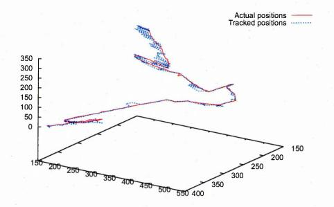
Figure 6.59: Comparison of the tracked positions and the manually determined positions of the pipette tip when using using the Canny edge detector with the second setting and the motion filter.
