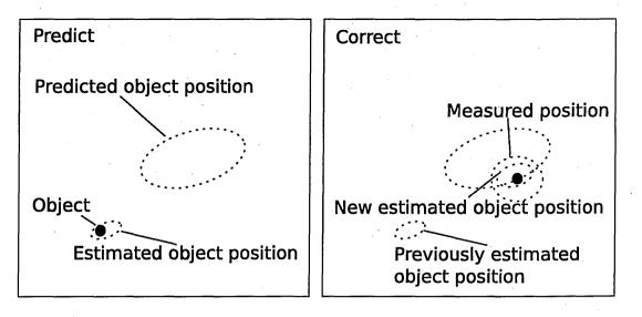
Figure 2.4: The Kalman filter can be divided into 2 stages
