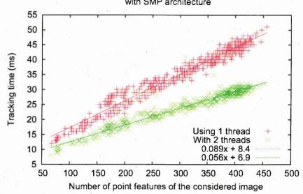
Comparison on a AMD Athlon MP 1600+ bi-processor computer with SMP architecture
