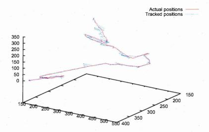
Figure 6.58: Comparison of the tracked positions and the manually determined positions of the pipette tip when using using the Canny edge detector with the first setting and the motion filter.
