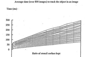
Figure 6.41: The same graph as in figure 6.39 but with a different viewpoint. This shows how the stencil decimation ratio affects the speed performance of the tracking
