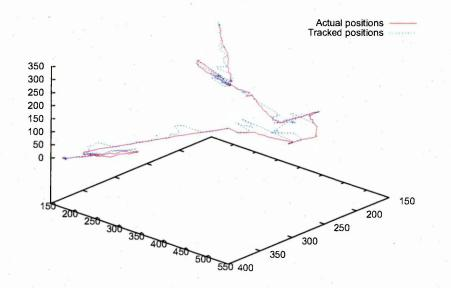
Figure 6.55: Comparison of the tracked positions and the manually determined positions of the pipette tip when using our custom edge detector.
