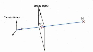
Figure B.2: By obtaining the intrinsic parameter it is possible to determine where each point expressed in the camera frame will be projected onto the image.
