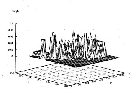
Figure 6.45: The heavy background clutter is illustrated by the existence of multiple peaks in the graph. In spite of the heavy clutter the pipette tip is well localised through further evaluation of the peak points.
