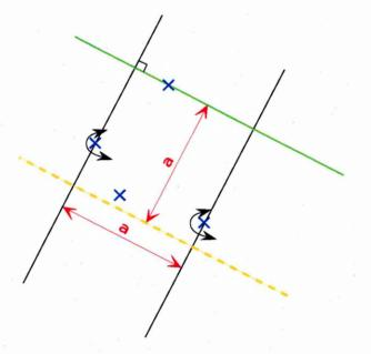
Figure A.9: 2 Points are taken randomly, by assuming that they belong to opposite edges, for instance, a system of equations can be written and solved to check if it is possible to construct squares that are intersecting this four points. Curved arrows represent the possible rotations of the parallel lines.
