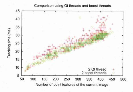
Figure 6.10: Comparison of Qt threads and boost threads, both implementation uses Qt mutexes
