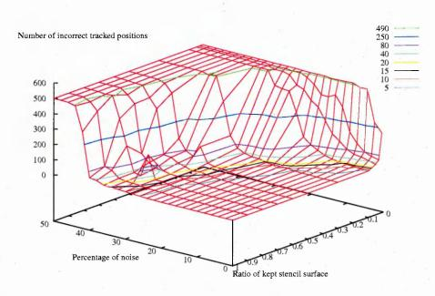
Figure 6.16: The z-axis corresponds to the number of images where the tracking result differs from the ground truth. The ratio of kept elements of the stencil is actually the ratio of the number of references listed in the 2-D array corresponding to the stencil elements kept. The colour lines outline error levels. This graph corresponds to the hand shape image sequences.
