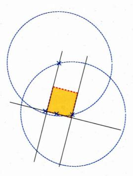
Figure A.5: It is not always possible to fit a square that intersects the 4 points using the assumption that the 2 points furthest apart belong to opposite edges and the 2 remaining points to one of the edge as shown with this configuration of four points.
