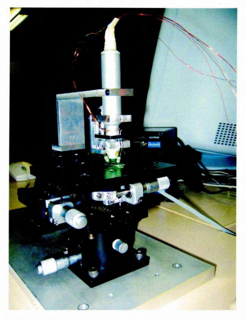
Figure 1.4: The set up at Sheffield Hallam university, the camera support is mounted on a piezo-electric three degree of freedom translation stage. Green LEDs are used to illuminate the scene. Green has been chosen to avoid interferences with the infrared communication of the MiCRoN robots. 1 pixel in the obtained image corresponds to 1 micrometre ( $\mu$ m).
