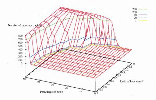
Figure 6.18: The z-axis corresponds to the number of images where the tracking result differs from the ground truth. The ratio of kept elements of the stencil is actually the ratio of the number of references listed in the 2-D array corresponding to the stencil elements kept. The colour lines outline error levels. This graph corresponds to the watch shape sequences
