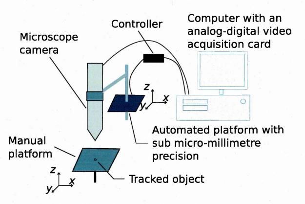
Figure 6.2: Diagram of the set-up used for the experiments. A photo of the set-up can be found figure 1.4, page 6.
