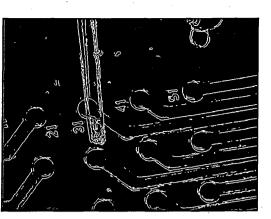
frame B: the same image filtered with the Canny edge detector.
