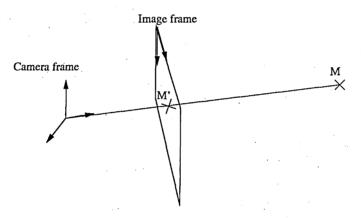
Figure 2.1: By obtaining the intrinsic parameter it is possible to determine where each point expressed in the camera frame will be projected onto the image.
