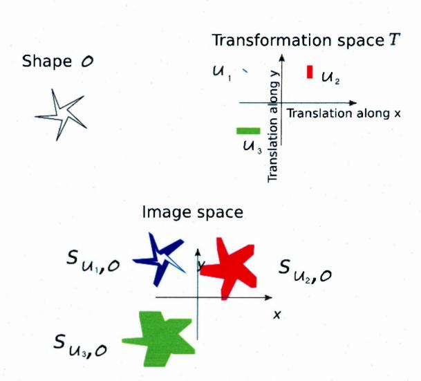
Figure 5.1: The stencils of the "star" shape corresponding to the coloured area of the transformation space have been drawn in the image space. The coloured regions are the set of points overlapped by the shape when it is moved according to the transformations of the subset having the same colour in the transformation space.
