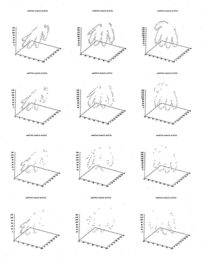
Figure 6.22: Stencils for the hand shape. The z-axis represents the number of overlapping stencils. Each row represents a different stencil decimation level corresponding to those of figure 6.20: 100%, 56%, 32%, 18%
