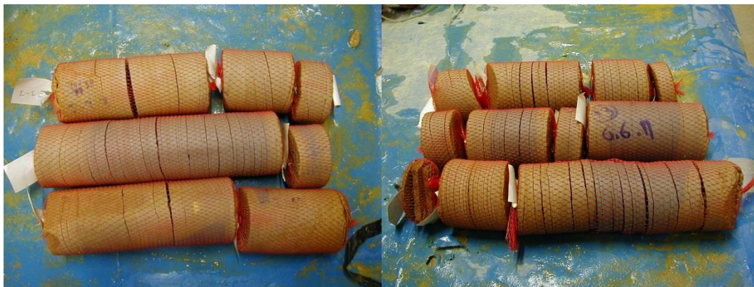
Figure 12 Typical progression of splitting at 10 cycles (left) and 20 cycles (right)
