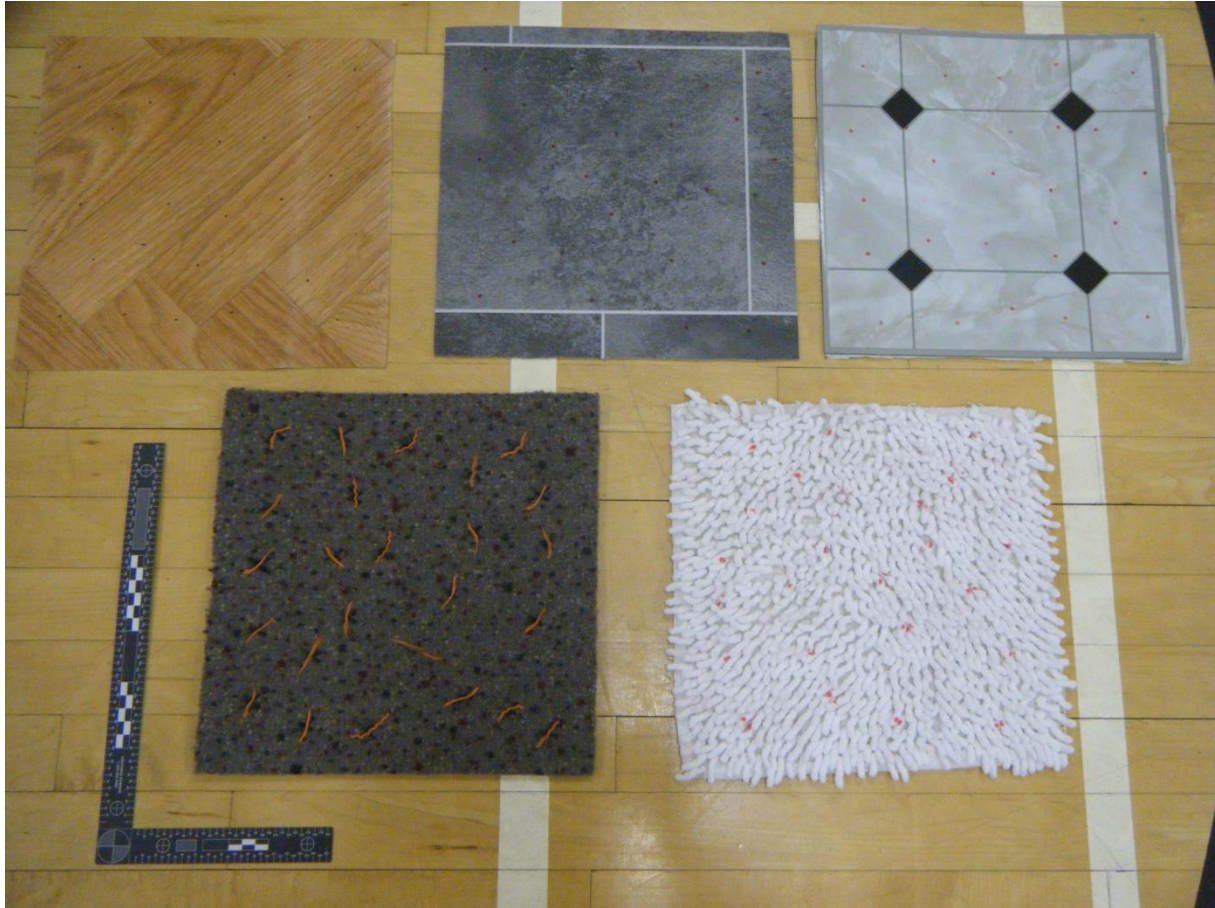
Figure 1. Floor surface sample tiles. (Left to right) top: smooth linoleum, rough linoleum and hard vinyl tile. Bottom: carpet tile and bath mat. The carpet tile is set up in the "before exposure" format with evidence placed on each marked point. The carpet tile's marked points were crosses to improve visual contrast with the tile's spotted pattern. All other tiles were marked with dots.
