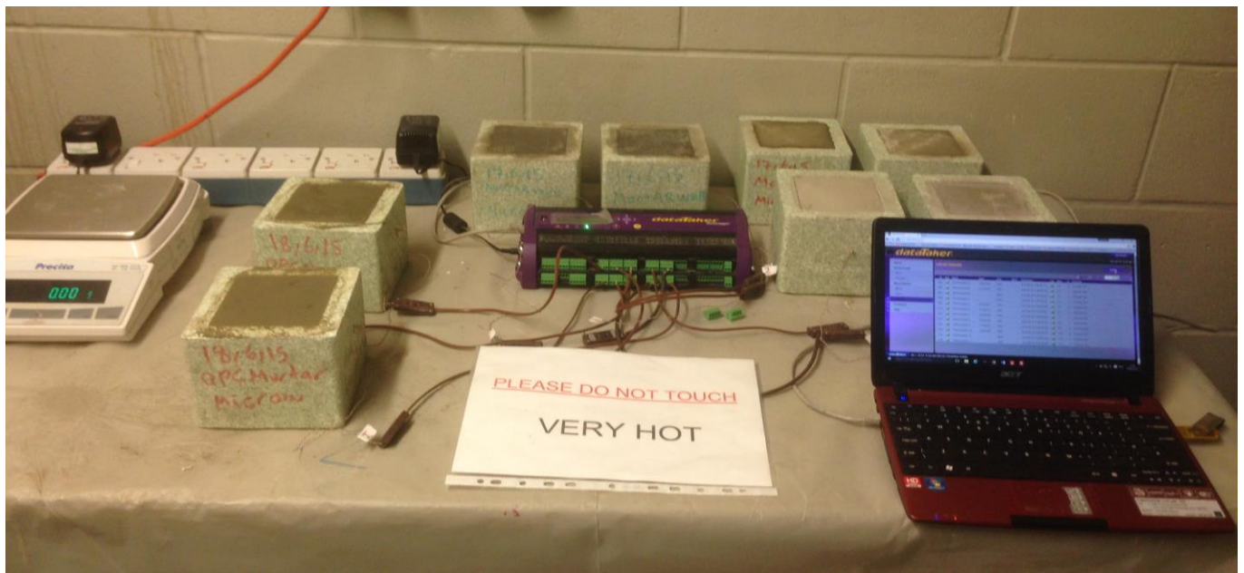
Figure 2. Set up for monitoring internal temperature
