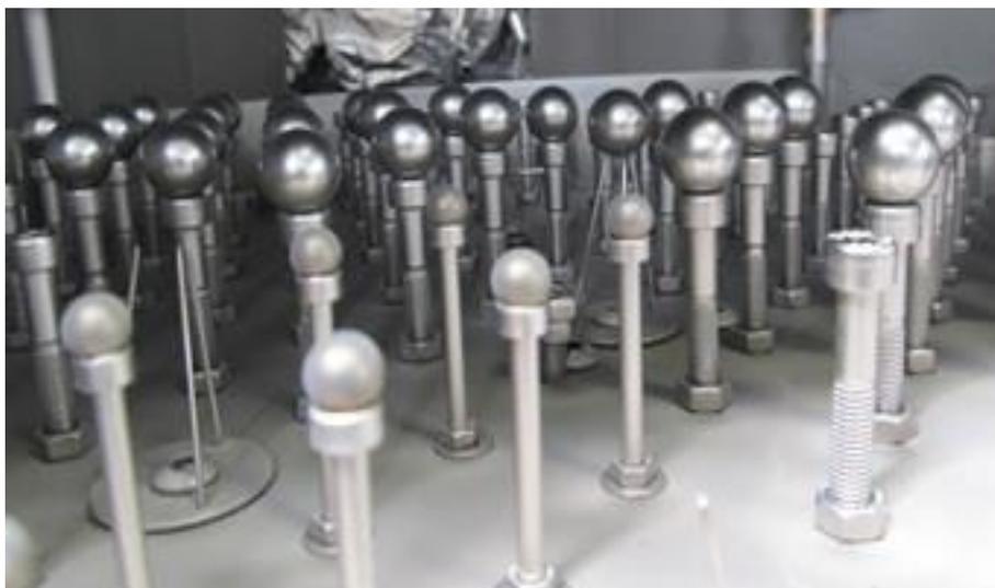
**Figure 1** A photograph taken inside the nitriding chamber, showing balls supported on the individual jigs.
