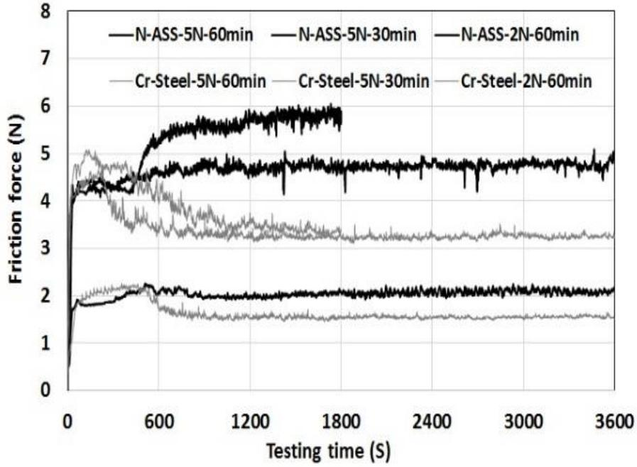
Figure 7 Friction curves of the tested samples.
