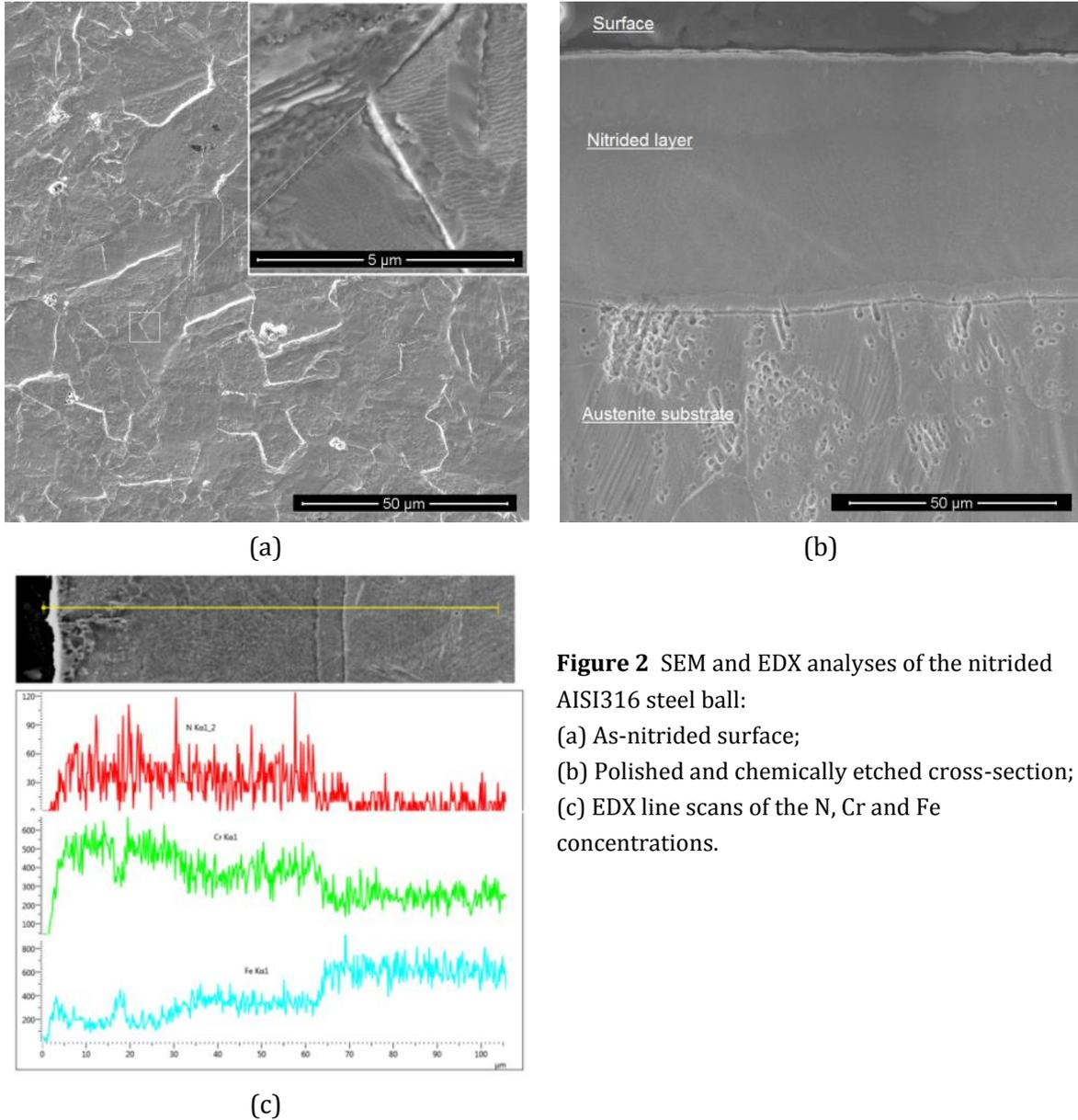
**Figure 2** SEM and EDX analyses of the nitrided AISI316 steel ball:
