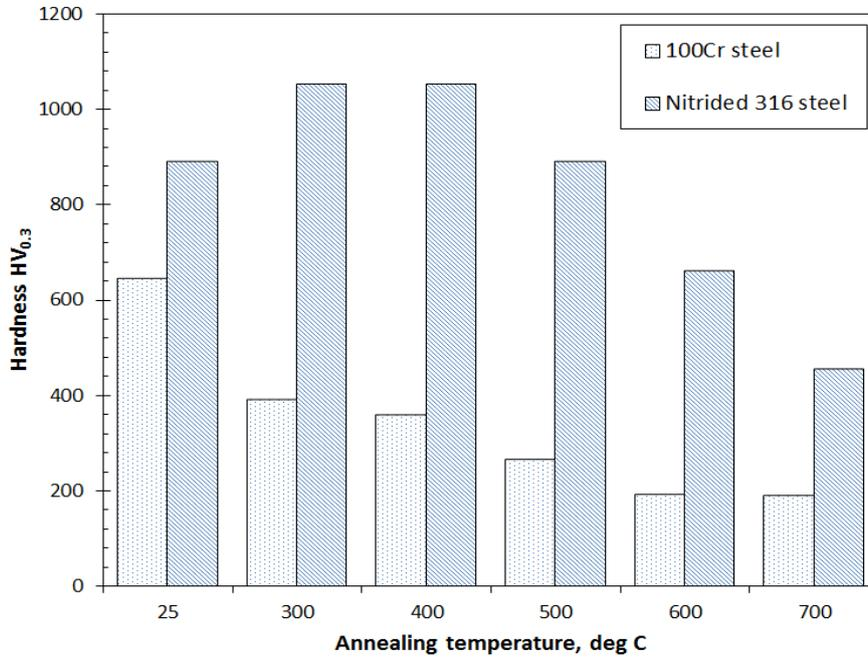
Figure 5. Effect of annealing temperature on the hardness property of nitrided 316 steel and hardened 100Cr steel.
