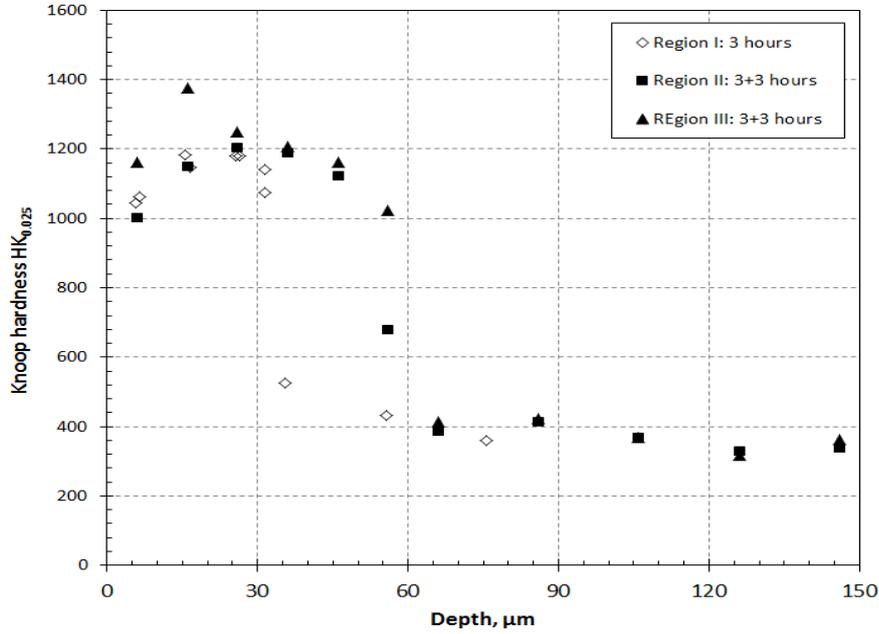
Figure 4. Microhardness depth profiles of as-nitrided ball.
