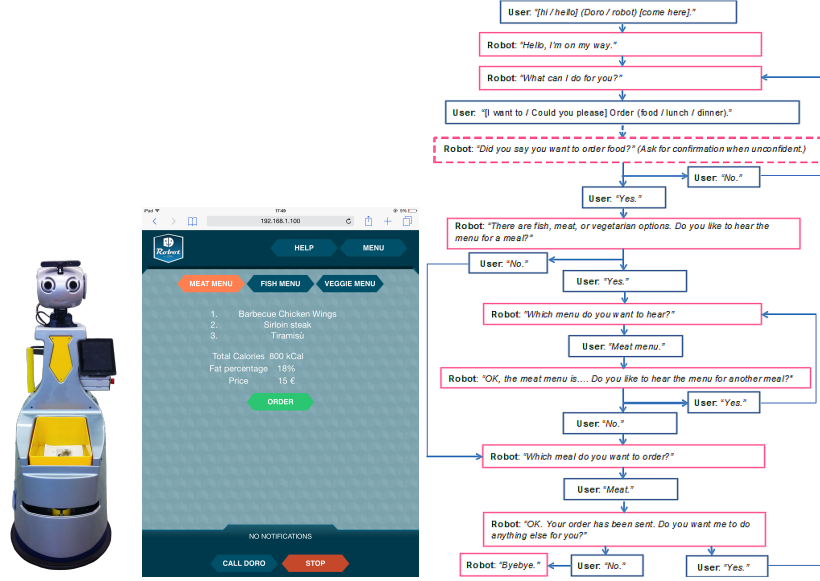
Fig. 1. (Left) The customized robotic platform used in our experiment. (Center) The food delivery page on the GUI. (Right) Dialogue flow (SUI) for the food delivery service.
