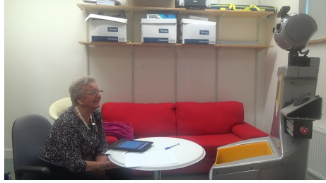
Fig. 2. Focused experiment in a controlled setting. The elderly participant is sitting in front of the robot, while the tablet is detached and placed on the table easy accessible by the user.
