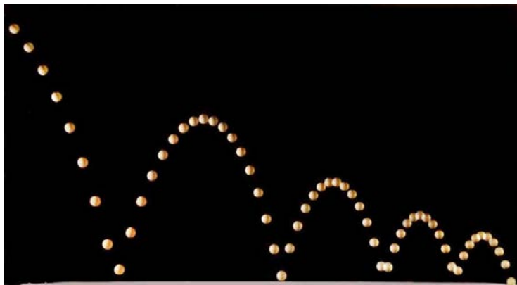
Fig. 1. Stroboscopic image of a ball bounce (image courtesy of Professor Andrew Davidhazy, Rochester Institute of Technology)
