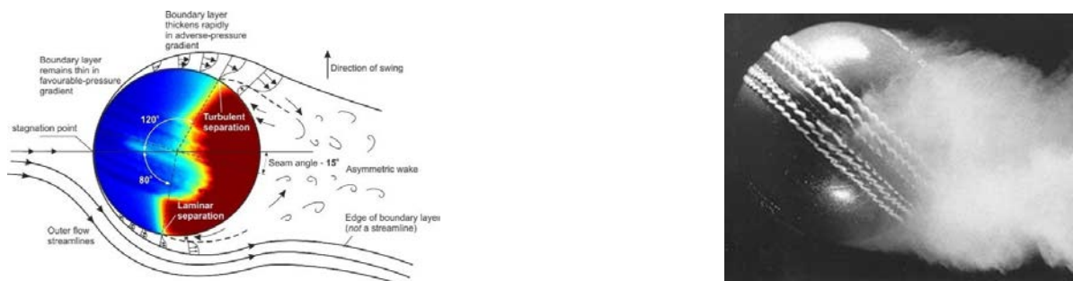
Fig. 4. Left: Infrared visualization technique to show separation points on a cricket ball (image courtesy of Dr James Scobie and Dr Gary Lock, University of Bath). Right: Smoke flow visualization over a cricket ball with the seam tripping the flow causing an asymmetric wake (image courtesy of Dr Rabi Mehta, Sports Aerodynamic Consultant).
