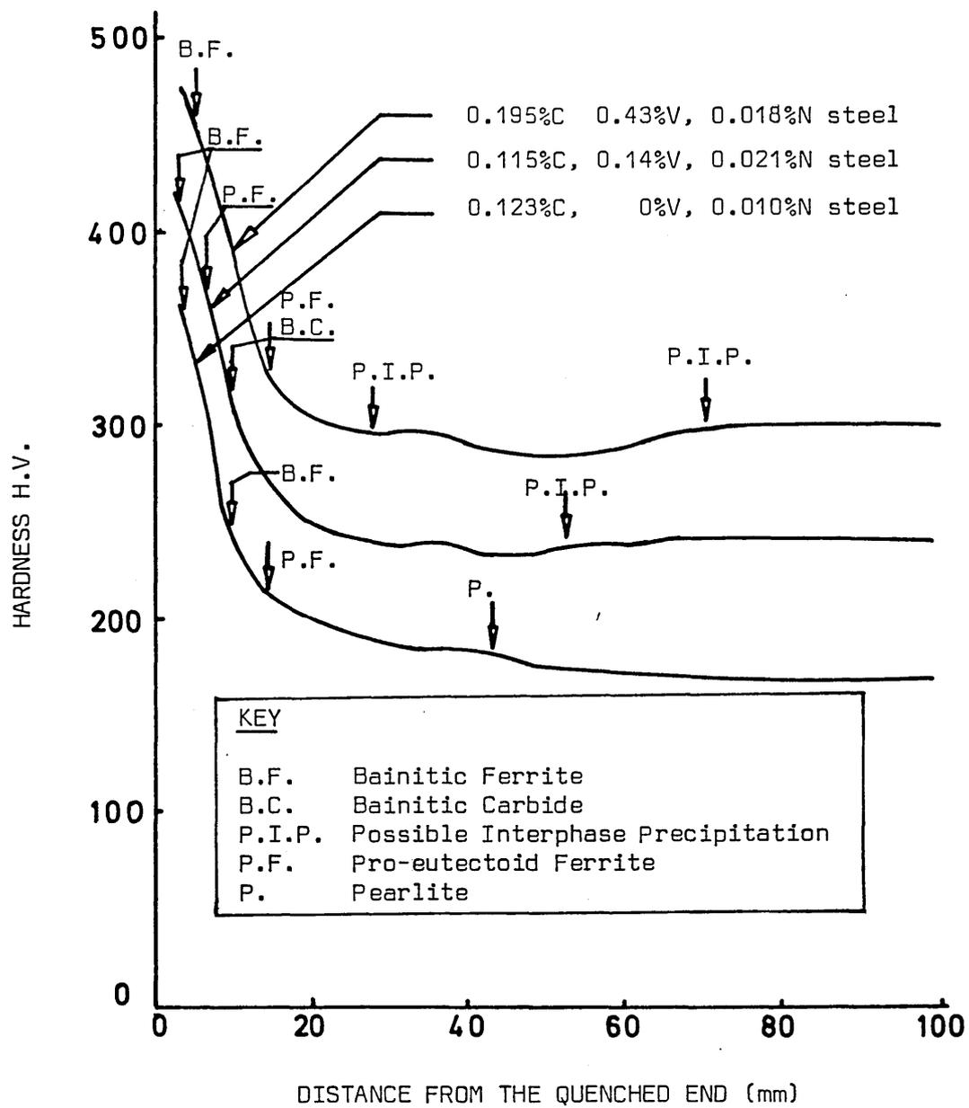
FIG. 76 EFFECT OF CARBON VANADIUM AND NITROGEN ON THE HARDENABILITY CURVES 1.6%Mn STEEL
