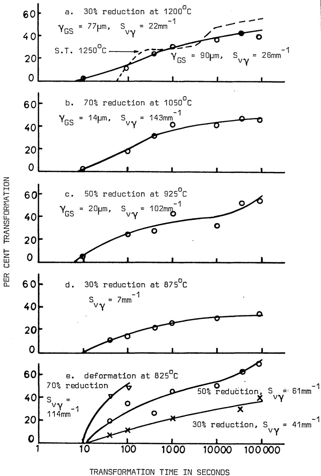
FIG. 97 EFFECT OF DEFORMATION PRIOR TO ISOTHERMAL TRANSFORMATION AT 750°C IN 0.12%C, 1.4/1.6%Mn, 0.13/0.19%V AND 0.010%N STEELS
