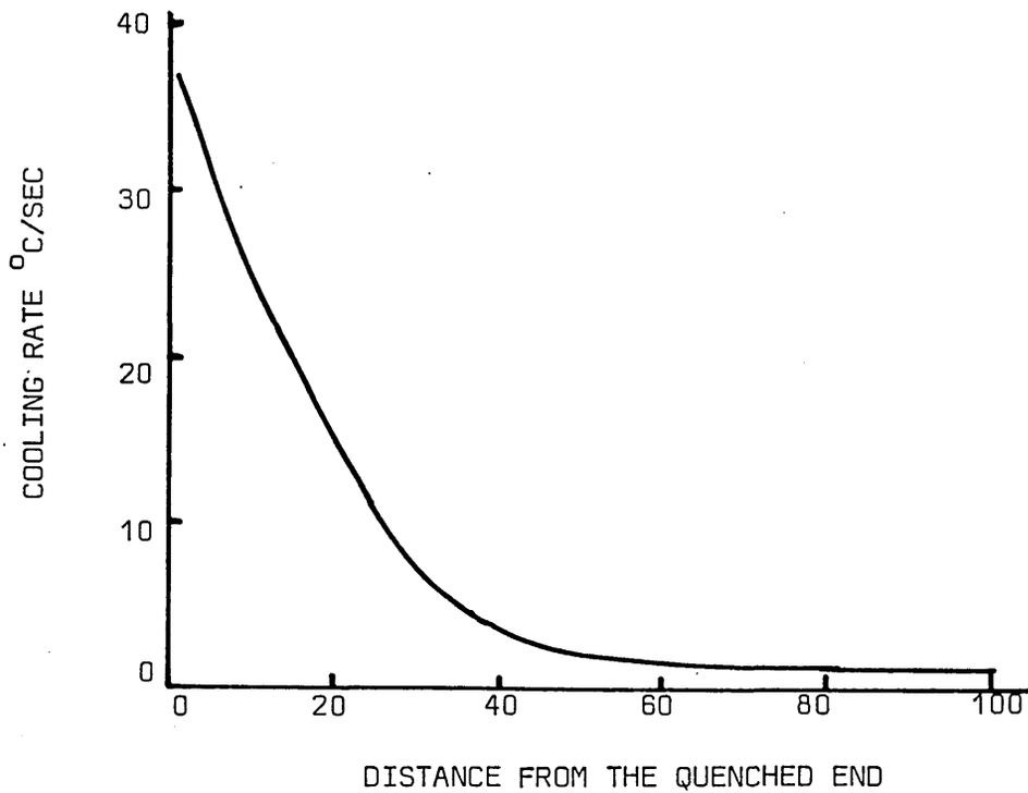
FIG. 75 RATE OF COOLING AS A FUNCTION OF DISTANCE FROM THE QUENCHED END OF MODIFIED JOMINY SPECIMEN
