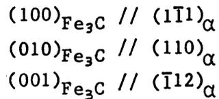
Because pearlite comprises interpenetrating single crystals of ferrite and cementite which have orientation relationships with the austenite grain into which they do not grow, they have mutual orientation relationship with each other. In eutectoid pearlite, forming on "clean" austenite grain boundaries in which there is no pro-eutectoid phase this is the Pitch/Petch orientation relationship<sup>(127)</sup>:-
