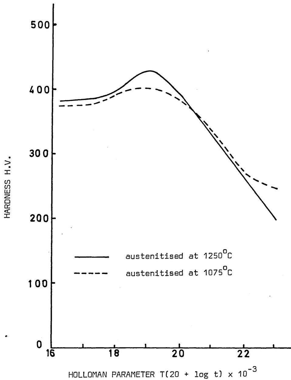
FIG. 56 EFFECT OF AUSTENITISING TEMPERATURE ON TEMPERING CURVES FOR QUENCHED 0.20%C, 0.45%V, 0.020%N STEEL
