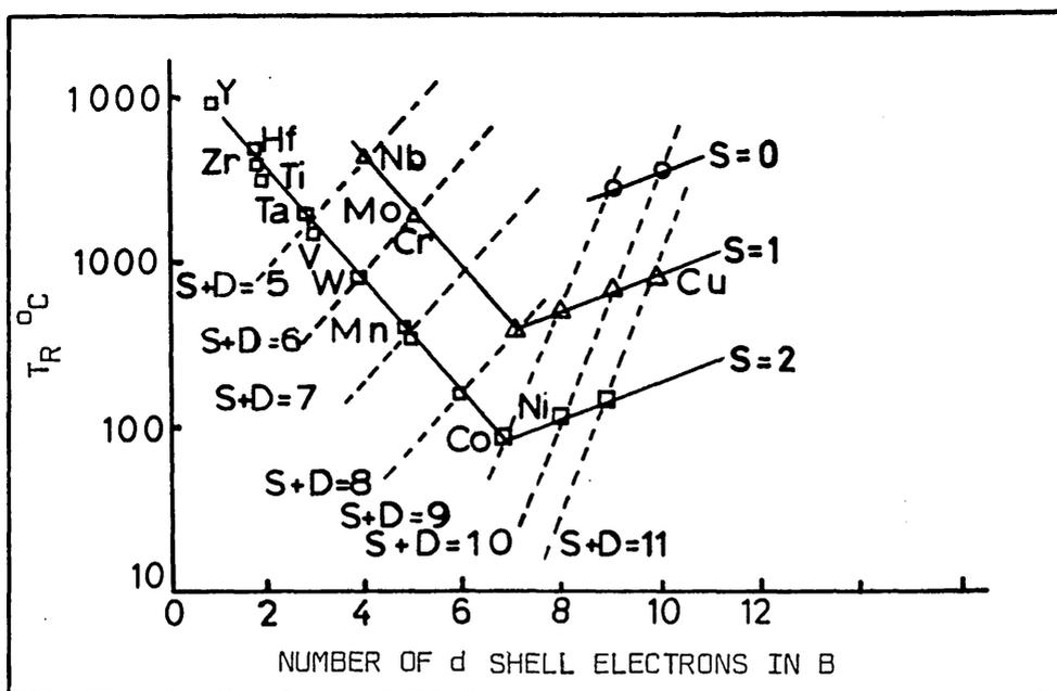
FIG. 12 RATE OF CHANGE OF RECRYSTALLISATION TEMPERATURE PER ATOMIC % SOLUTE ELEMENT ( $T_R$ ) IN IRON AS A FUNCTION OF THE NUMBER OF OUTERSHELL ELECTRONS OF THE SOLUTE ELEMENT.
