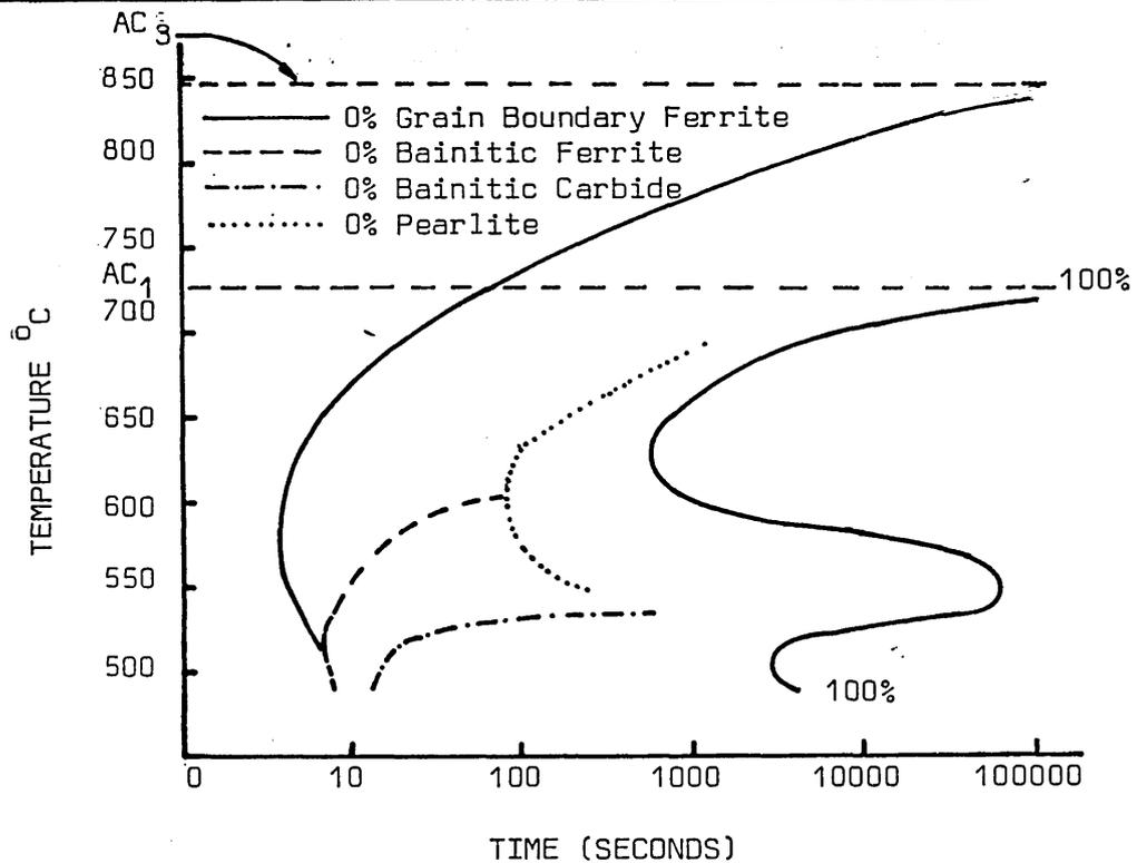
FIG. 63 ISOTHERMAL TRANSFORMATION DIAGRAM FOR 0.12%C, 1.58%Mn, 0.13%V, 0.01%N STEEL AUSTENITISED AT 1250°C, AUSTENITE GRAIN SIZE 90 μm
