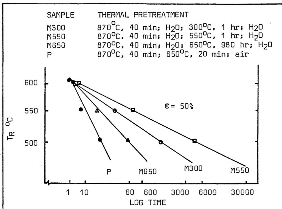
FIG. 16 TIME TO INITIATION OF RECRYSTALLISATION AS A FUNCTION OF TEMPERATURE  $T_R$  AND PRETREATMENT MT. AMOUNT OF COLD WORK  $\epsilon = 50\%$
