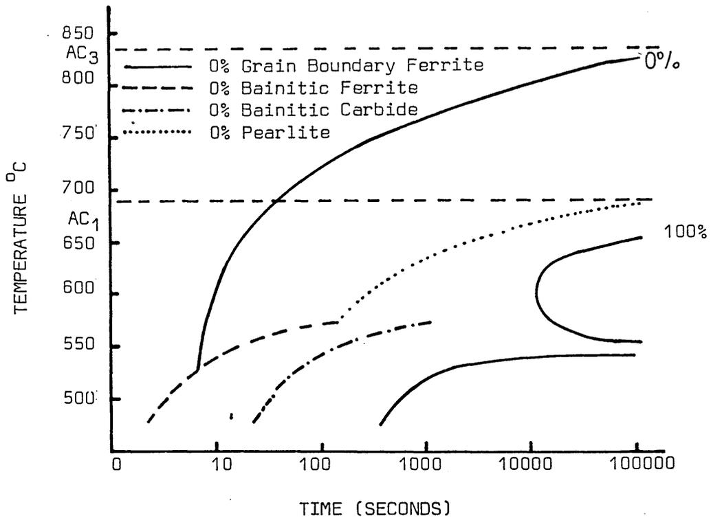
FIG. 62 ISOTHERMAL TRANSFORMATION DIAGRAM FOR 0.123%C, 1.6%Mn, 0.01%N STEEL AUSTENITISED 1250°C, AUSTENITE GRAIN SIZE 175 μm
