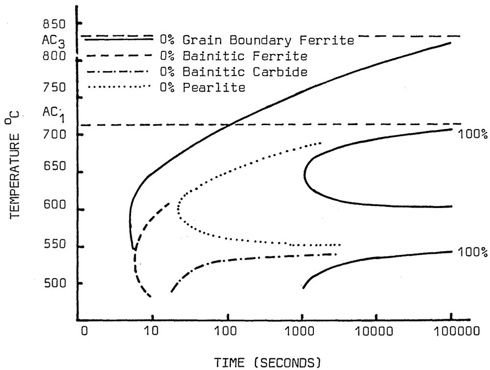
FIG. 66 ISOTHERMAL TRANSFORMATION DIAGRAM FOR 0.11%C, 1.66%Mn, 0.14%V, 0.005%N, AUSTENITISED AT 1250°C, AUSTENITE GRAIN SIZE 198 μm
