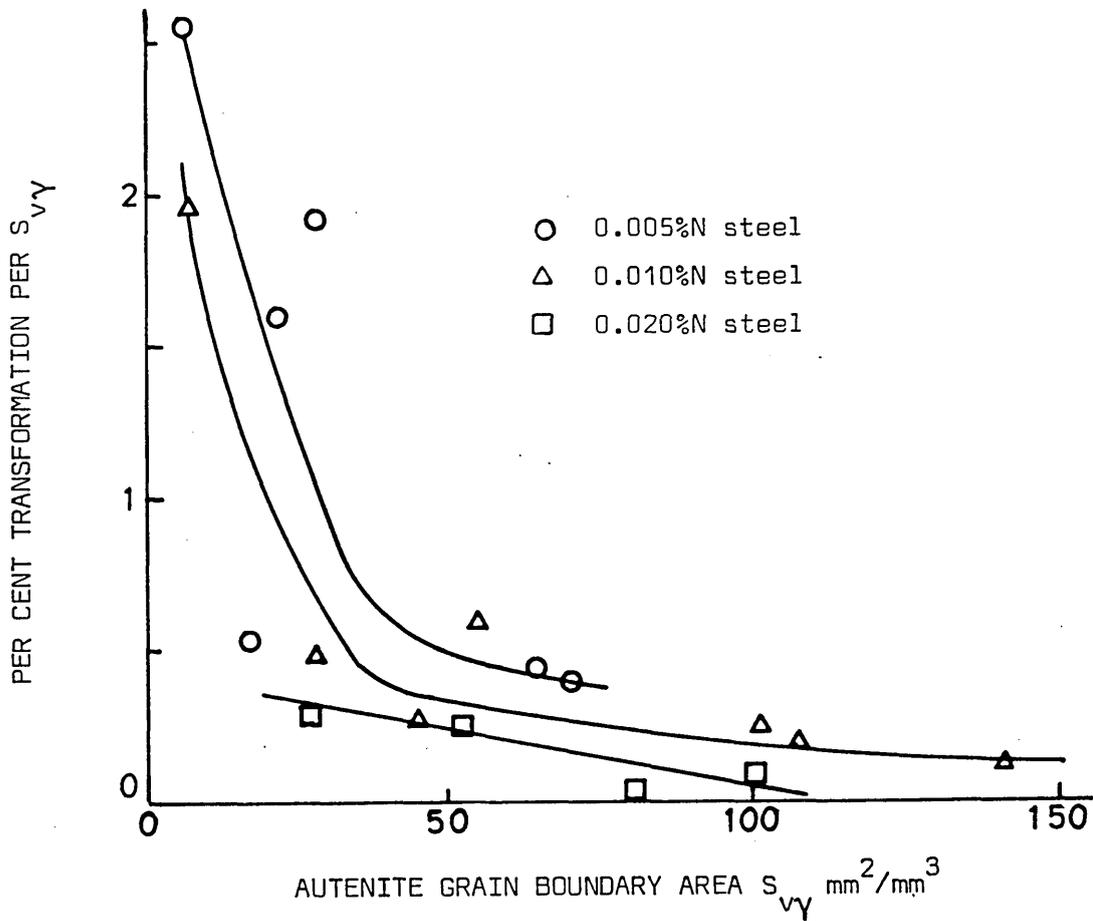
FIG. 106 EFFECT OF NITROGEN ON THE  $S_{v\gamma}$  ON TRANSFORMATION AT 750°C FOR 100 SECONDS
