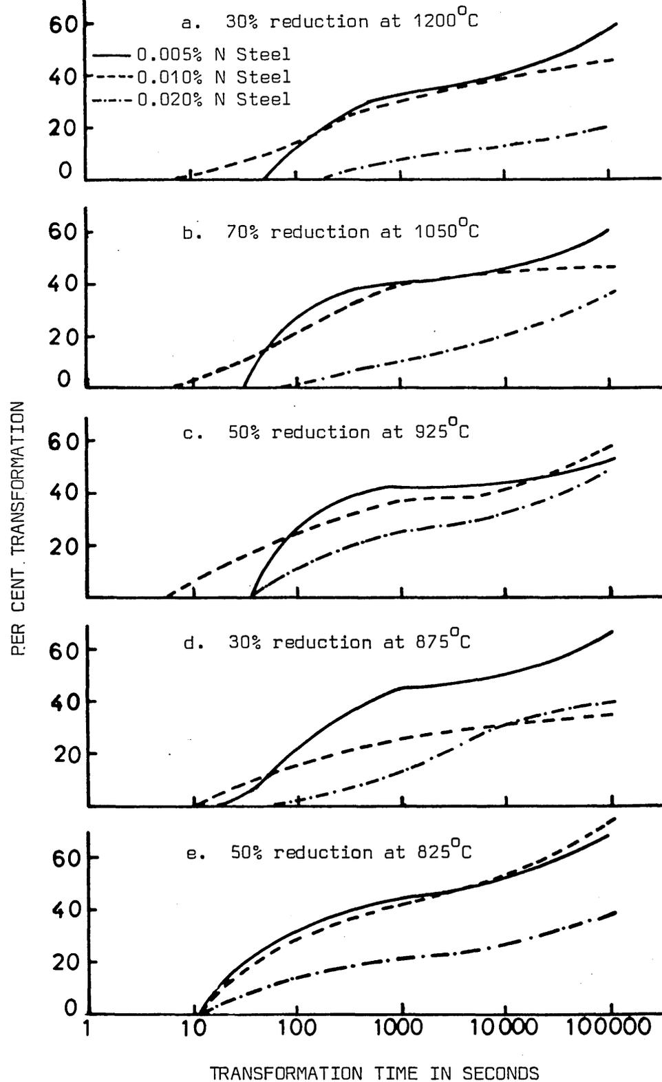
FIG. 105 EFFECT OF NITROGEN ON THE ISOTHERMAL TRANSFORMATION AT 750°C IN 0.12/0.128%C, 1.4/1.8%Mn AND 0.13/0.19%V STEELS
