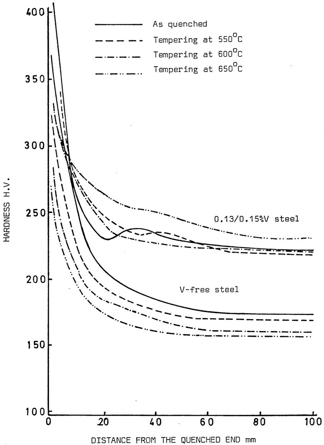
FIG. 78 TEMPERING OF JOMINY BARS IN V-FREE 0.128%C, 1.70%Mn, 0.0075%N STEEL AND 0.12%C, 0.13/0.15%V, 1.60%Mn, 0.010%N STEEL AFTER AUSTENITISING AT 1075°C
