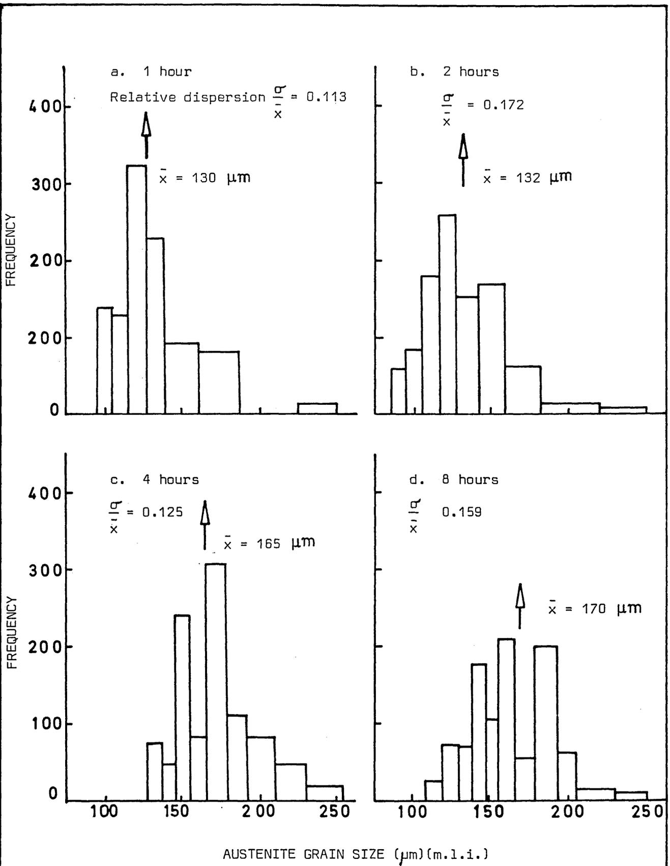
FIG. 44 AUSTENITE GRAIN GROWTH AFTER AUSTENITISING AT 1050°C UP TO 8 HOURS IN 0.113%C, 0.14%V, 0.005%N STEEL
