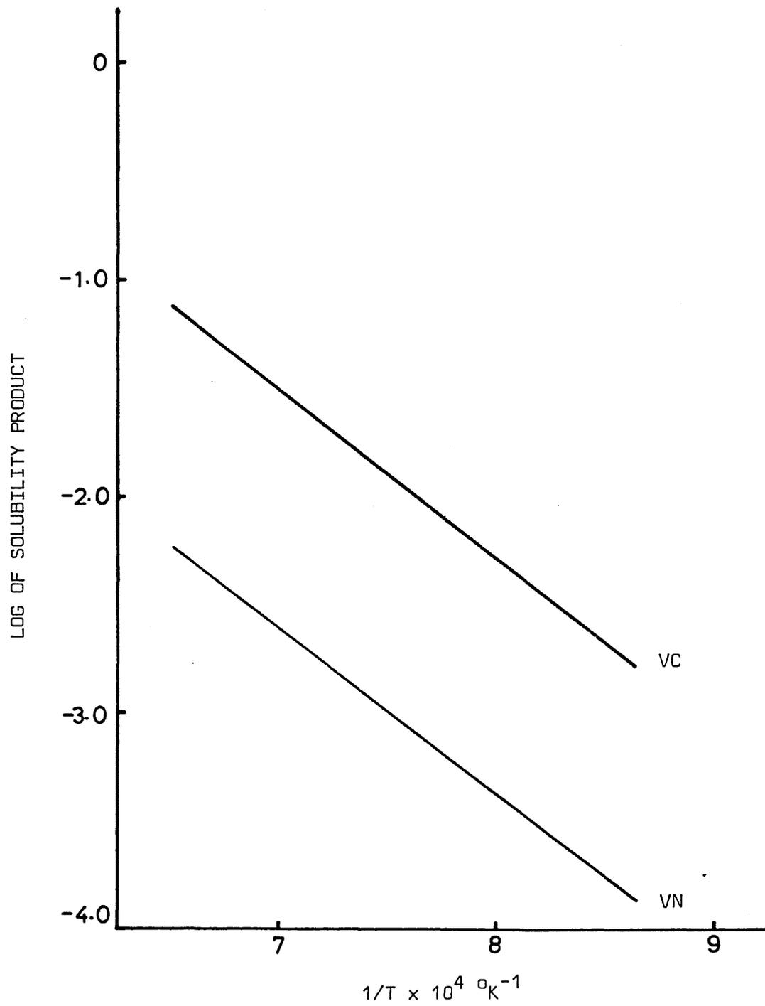
FIG. 38 SOLUBILITY PRODUCT - TEMPERATURE RELATIONSHIP OF VANADIUM-CARBIDE AND VANADIUM NITRIDE IN 0.126%C, 1.77%Mn, 0.415%V, 0.020%N STEEL
