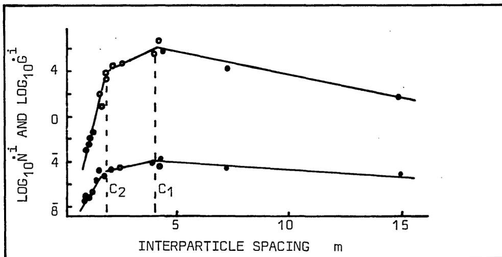
FIG. 14 APPARENT NUCLEATION  $\dot{N}$  AND GROWTH  $\dot{G}$  RATE AS A FUNCTION OF INTERPARTICLE SPACING FOR Al-Cu ALLOYS (o) AND Al-Fe ALLOYS (●)  $C_1 = 4 \mu\text{m}$ ,  $C_2 = 1.8 \mu\text{m}$ .
