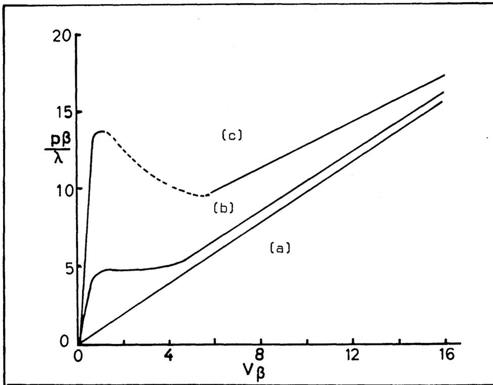
FIG. 11 THE DRIVING FORCE FOR GRAIN BOUNDARY MIGRATION AS A FUNCTION OF THE BOUNDARY VELOCITY. CURVE (a) REPRESENTS A PURE METAL. CURVES (b) AND (c) REPRESENTS SOLID SOLUTION ALLOYS OF INCREASING SOLUTE CONTENT.
