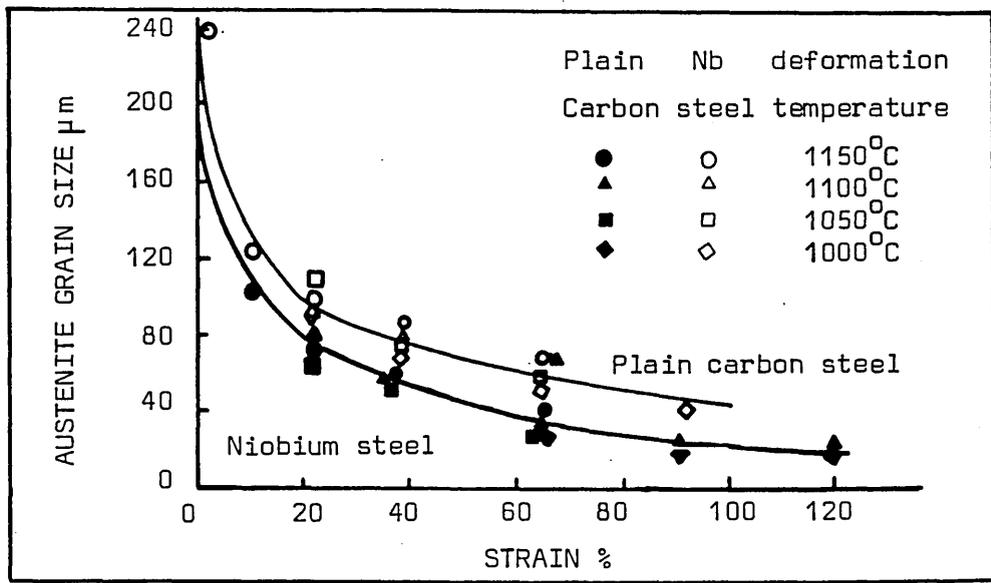
FIG. 18 INFLUENCE OF THE AMOUNT OF SINGLE-PASS DEFORMATION AND DEFORMATION TEMPERATURE ON RECRYSTALLISED AUSTENITE GRAIN SIZE IN PLAIN CARBON AND NIOBIUM STEELS
