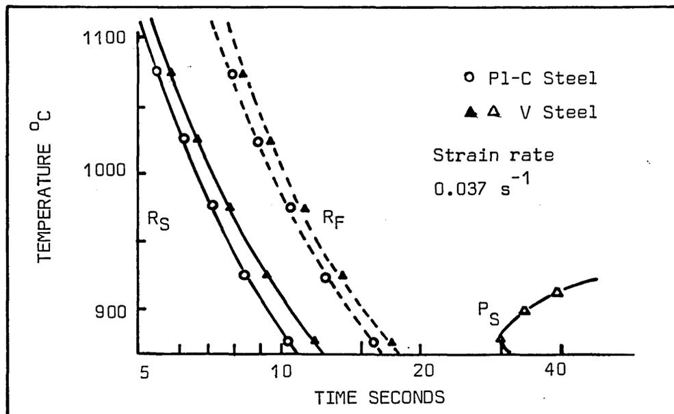
FIG. 22 DYNAMIC RECRYSTALLISATION AND DYNAMIC PRECIPITATION TIME TEMPERATURE DIAGRAM
