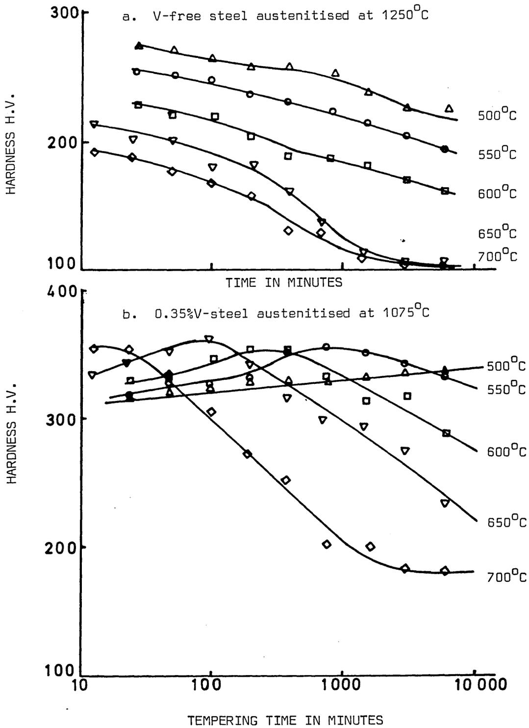
FIG. 51 ISOTHERMAL TEMPERING CURVES FOR 0.10%C, 1.50/1.60%Mn, 0.005/0.006%N STEEL
