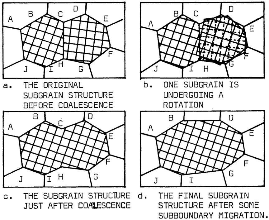
FIG. 3 SCHEMATIC REPRESENTATION OF SUBGRAIN COALESCENCE BY SUBGRAIN ROTATION.
