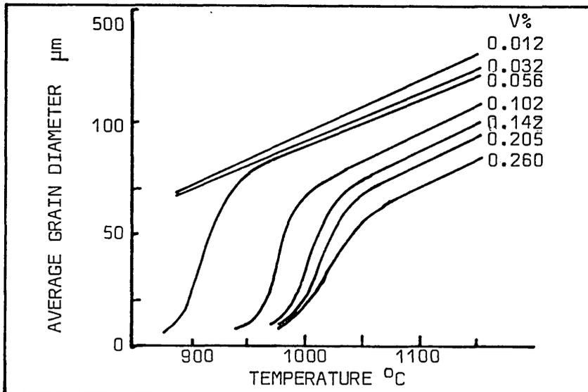
FIG. 26 AVERAGE AUSTENITIC GRAIN DIAMETER OF 0.2% C STEEL CONTAINING VARYING AMOUNTS OF VANADIUM.
