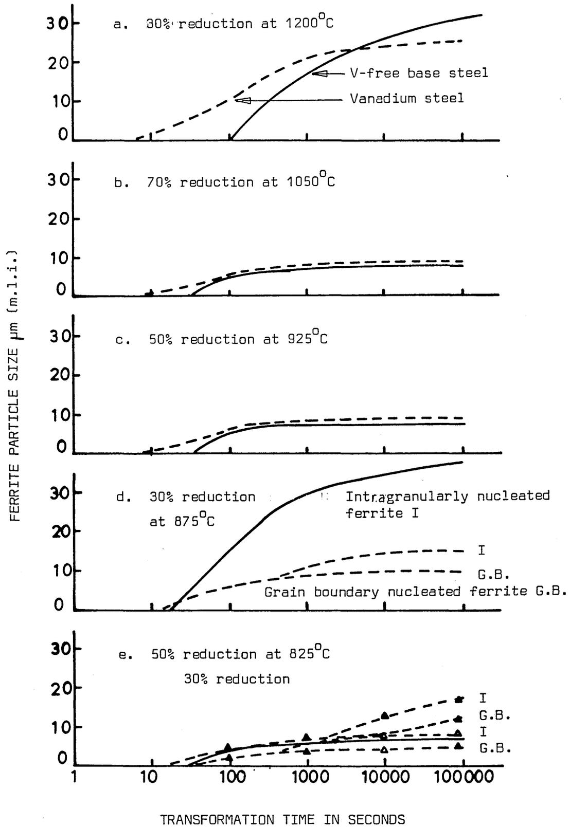
FIG. 100 EFFECT OF 0.13/0.19%V ADDITION ON THE FERRITE PARTICLE SIZE DURING ISOTHERMAL TRANSFORMATION AT 750°C IN 0.12%C, 1.4/1.7%Mn AND 0.010%N STEELS
