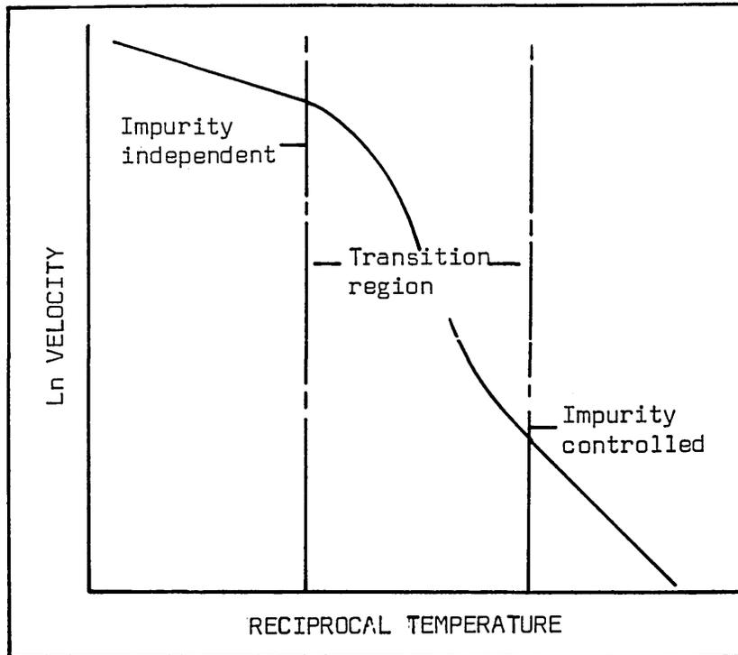
FIG. 9. SCHEMATIC REPRESENTATION OF THE EFFECT OF THE TEMPERATURE ON THE GRAIN-BOUNDARY VELOCITY ( $V$ ) DURING PRIMARY RECRYSTALLISATION.
