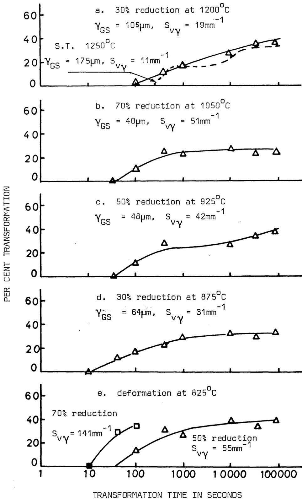
FIG. 94 EFFECT OF DEFORMATION PRIOR TO ISOTHERMAL TRANSFORMATION AT 750°C IN 0.12%C, 1.60/1.70%Mn, AND 0.0075/0.01%N STEELS
