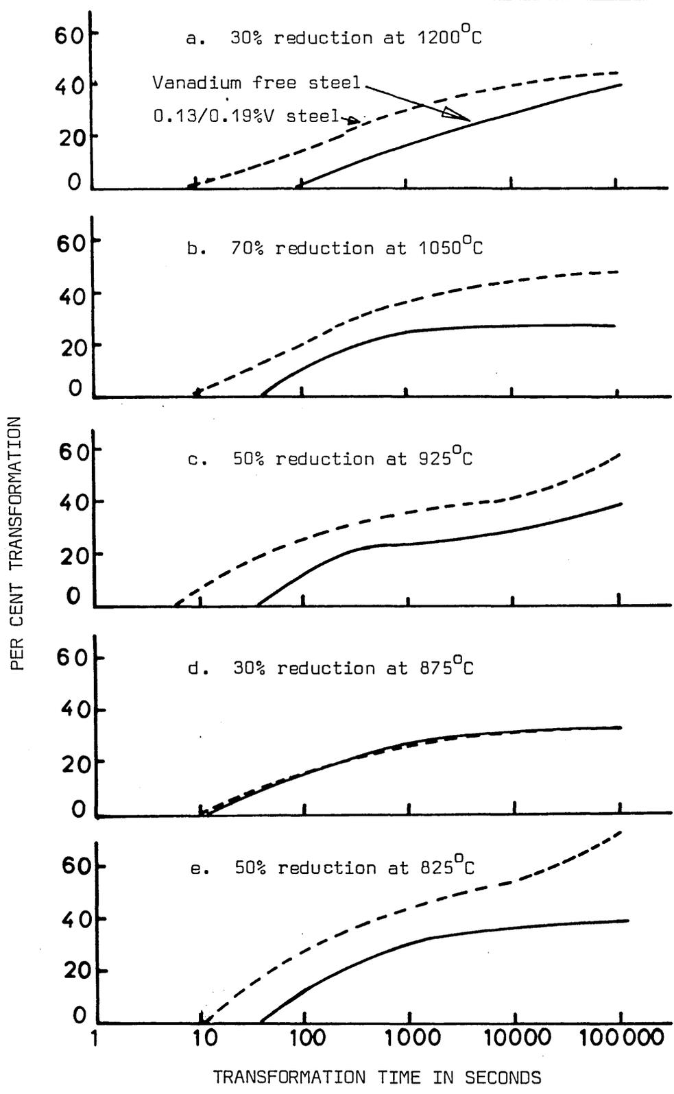
FIG. 99 EFFECT OF 0.13/0.19%V ADDITION ON THE ISOTHERMAL TRANSFORMATION AT 750°C IN 0.12/0.13%C, 1.4/1.7%Mn AND 0.010%N STEELS
