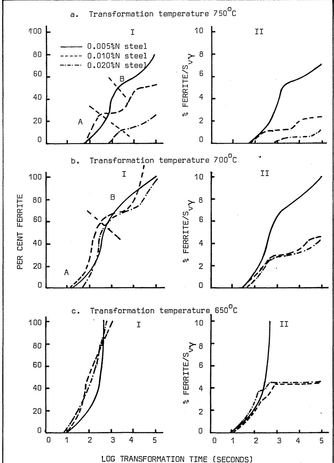
FIG. 61 EFFECT OF INCREASING NITROGEN ON THE FERRITE FORMATION IN 0.11/0.12%C, 1.6/1.8%Mn, 0.13/0.15%V STEELS
