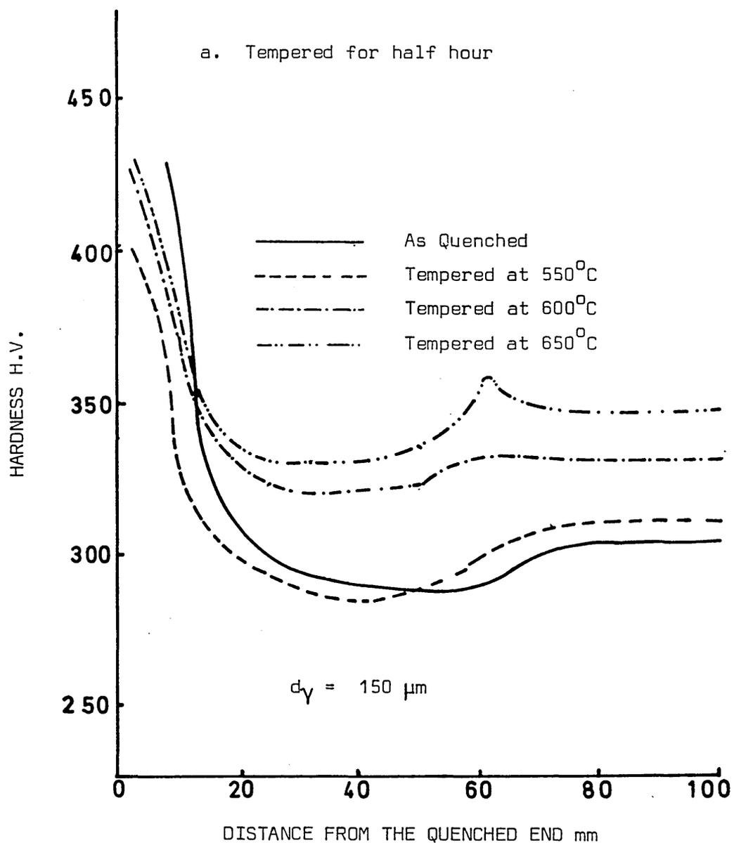
FIG. 82 MODIFIED JOMINY HARDNESS CURVES FOR 0.195% C,
