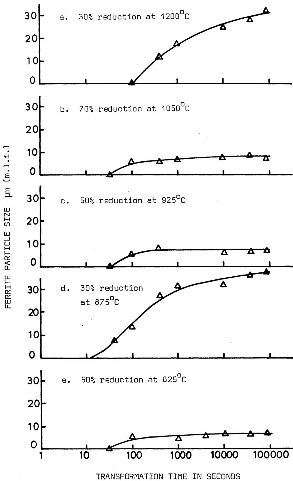
FIG. 96 EFFECT OF DEFORMATION PRIOR TO ISOTHERMAL TRANSFORMATION AT 750°C ON THE FERRITE PARTICLE SIZE IN 0.12%C, 1.60/1.70%Mn AND 0.0075/0.010%N STEELS
