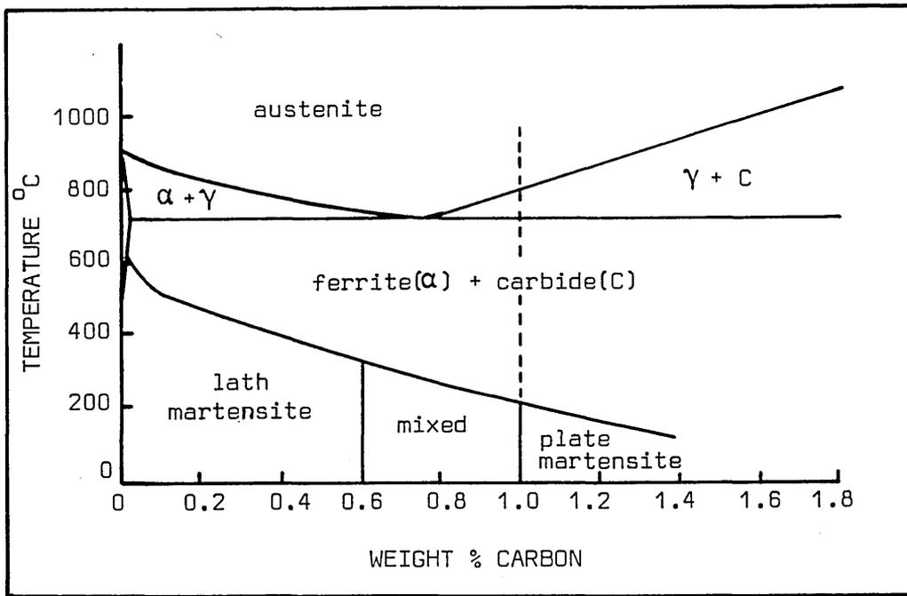
FIG. 27 RANGES OF LATH AND PLATE MARTENSITE FORMATION IN IRON CARBON ALLOYS
