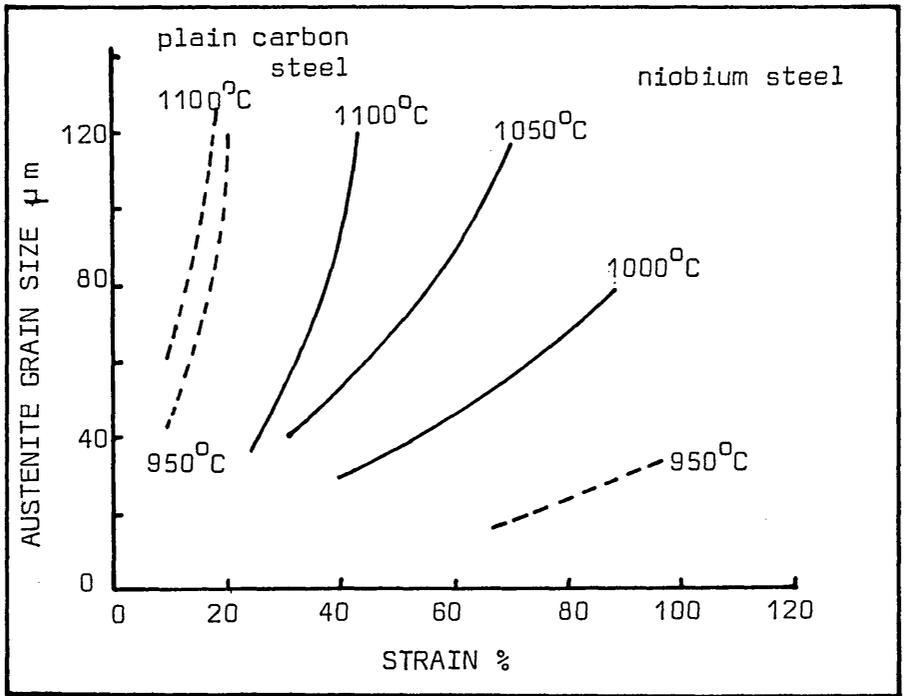
FIG. 19 EFFECT OF DEFORMATION TEMPERATURE AND INITIAL GRAIN SIZE ON CRITICAL AMOUNT OF DEFORMATION REQUIRED FOR COMPLETION OF RECRYSTALLISATION IN THE PLAIN CARBON AND NIOBIUM STEELS.
