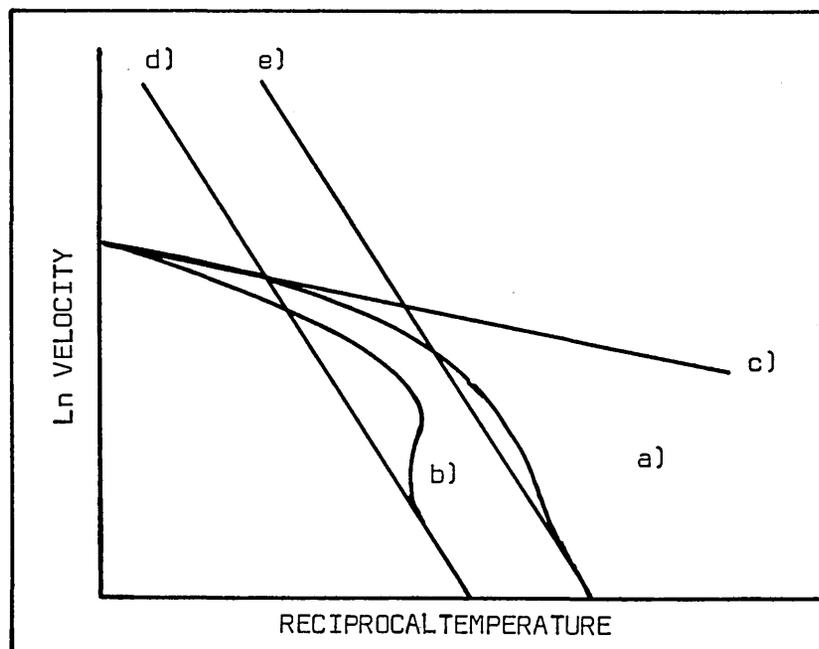
FIG. 10. SCHEMATIC REPRESENTATION OF THE GRAIN BOUNDARY VELOCITY ( $V$ ) AS A FUNCTION OF TEMPERATURE ( $T$ ) FOR TWO SOLUTE CONTENTS (a b), CURVE c REPRESENTS A BOUNDARY HAVING NO SOLUTE ATMOSPHERE. CURVES d AND e REPRESENT THE LIMITING CASES IN EQUATION 11.
