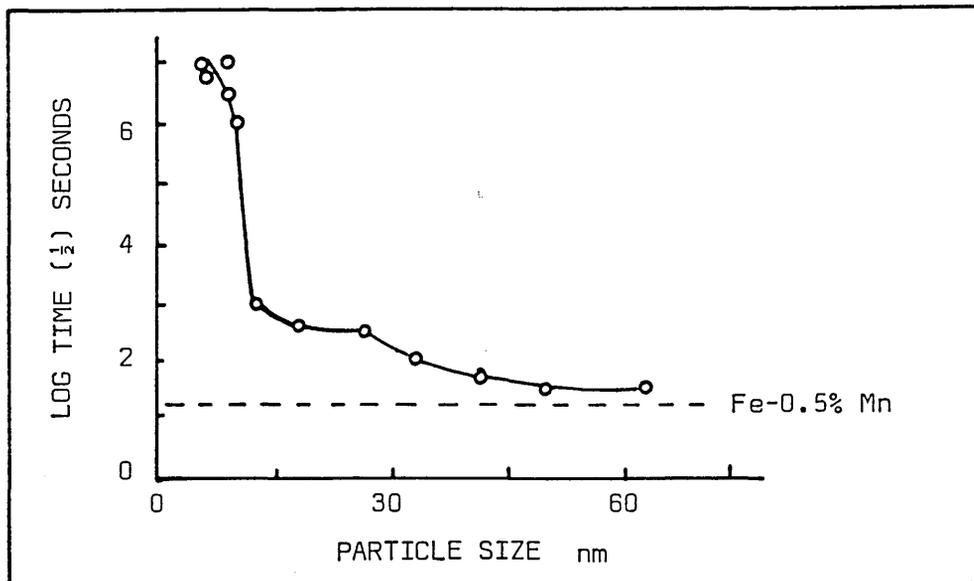
FIG. 15 THE TIME FOR 50% RECRYSTALLISATION AS A FUNCTION OF PARTICLE SIZE.
