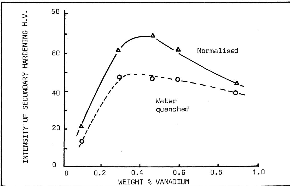
FIG.31 THE EFFECT OF VANADIUM ON THE INTENSITY OF SECONDARY HARDENING
