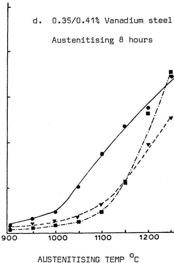
FIG. 47 EFFECT OF NITROGEN IN 0.10/0.126%C, 1.4/1.8%Mn STEEL ON THE GRAIN COARSENING CHARACTERISTICS OF AUSTENITE
