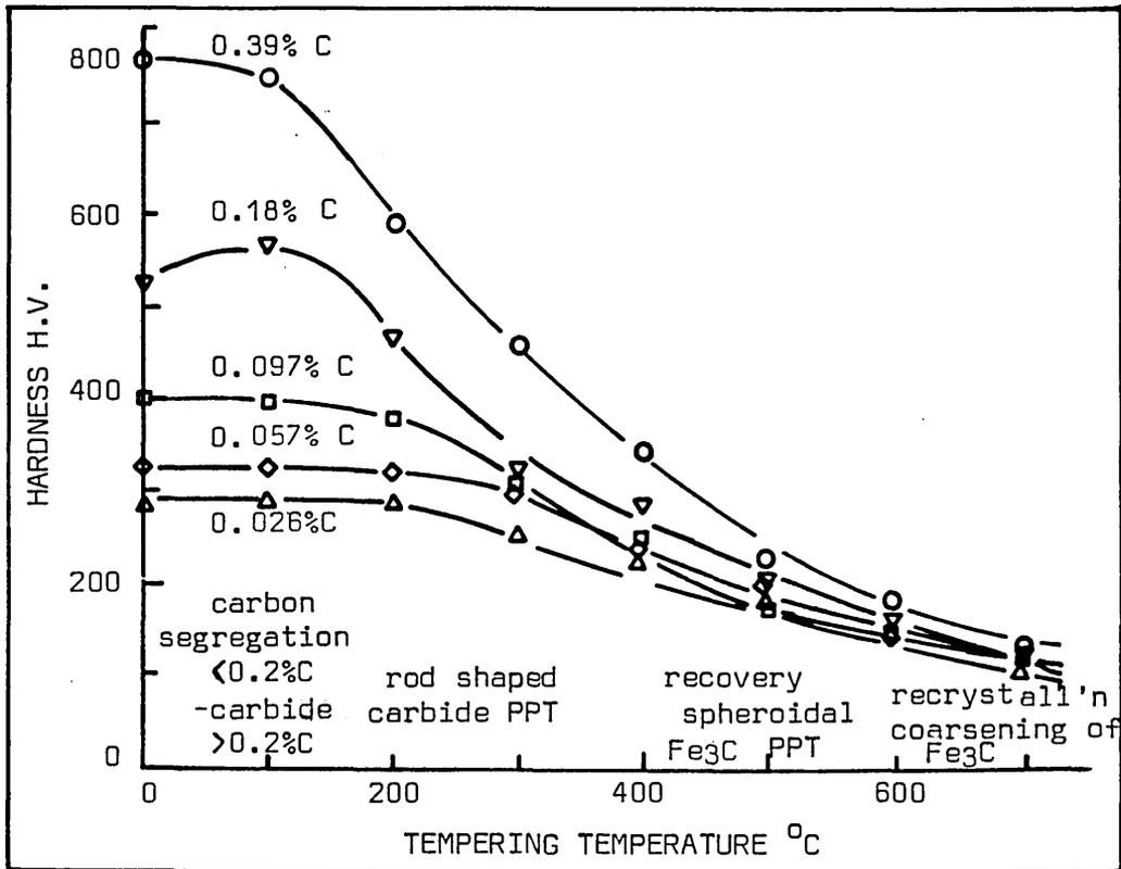
FIG. 28 HARDNESS OF IRON-CARBON MARTENSITES TEMPERED ONE HOUR AT 100-700°C
