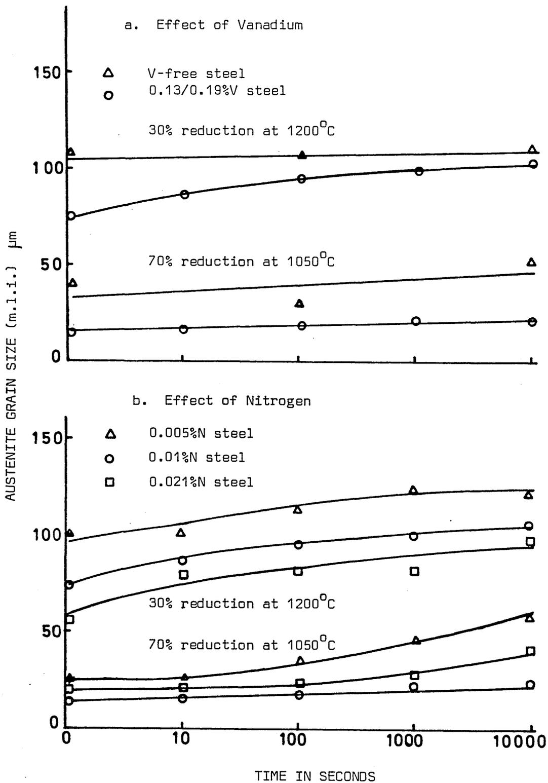
FIG. 89 EFFECT OF VANADIUM AND NITROGEN ON THE GRAIN COARSENING CHARACTERISTICS AT 925<sup>o</sup>C
