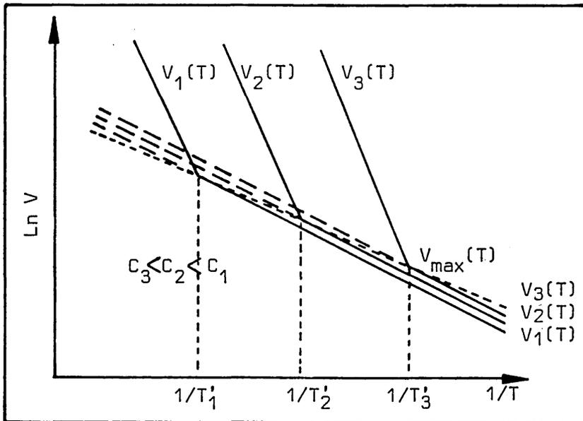
FIG. 8 SCHEMATIC REPRESENTATION OF THE TEMPERATURE DEPENDENCE OF THE GRAIN-BOUNDARY VELOCITY ( $V$ ) FOR VARIOUS SOLUTE CONCENTRATIONS ( $C$ ) DURING PRIMARY RECRYSTALLISATION.
