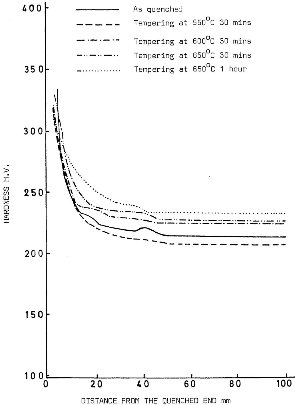
FIG. 79 EFFECT OF TEMPERING OF JOMINY BARS FOR 0.12%C, 0.13/0.15%V, 0.010%N STEEL AFTER AUSTENITISING AT 1250°C
