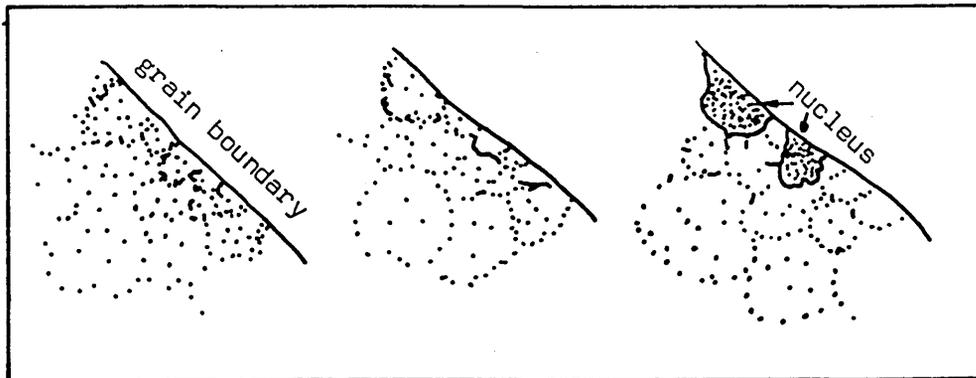
FIG. 2 NUCLEATION AND SUBGRAIN GROWTH (SCHEMATIC). SUBGRAIN BOUNDARIES THICKLY POPULATED BY DISLOCATIONS (DOTS) HAVE A HIGH MISORIENTATION ANGLE AND ARE MOST LIKELY TO MIGRATE.
