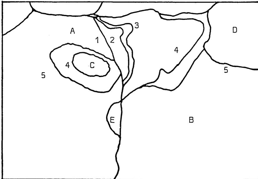
FIG. 6 OUTLINE OF A MICROGRAPH SHOWING STRAIN-INDUCED BOUNDARY MIGRATION. STRAIN INDUCED GROWTH OF A AT THE EXPENSE OF B. DIFFERENT ANNEALING TIMES CAUSED THE BOUNDARY TO MIGRATE AT (1<2<3<4<5) LONGER ANNEALING TIMES. C, D AND E RECRYSTALLISED GRAINS.
