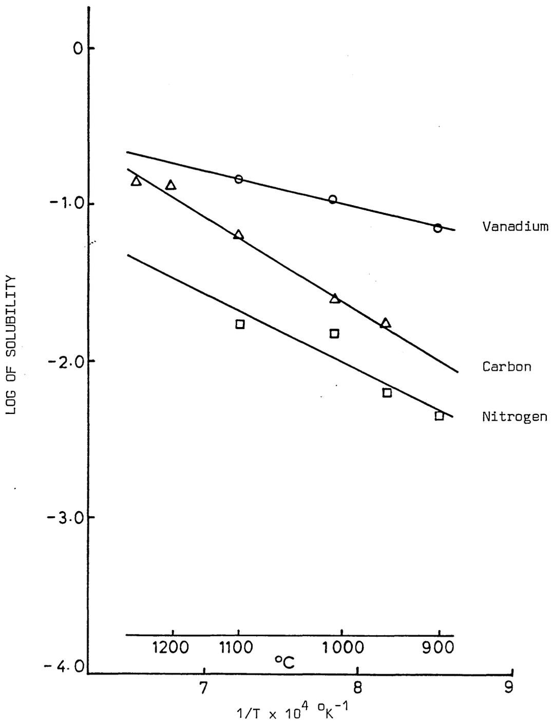
FIG. 36 EFFECT OF SOLUTION TREATMENT TEMPERATURE ON THE SOLUBILITY OF VANADIUM, CARBON AND NITROGEN IN 0.212%C 1.83%Mn 0.14%V 0.018%N STEEL
