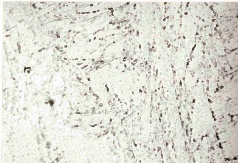
FIG. 53 TEMPERED MICROSTRUCTURES OF 0.12% C, 1.77% Mn, 0.15% V,
