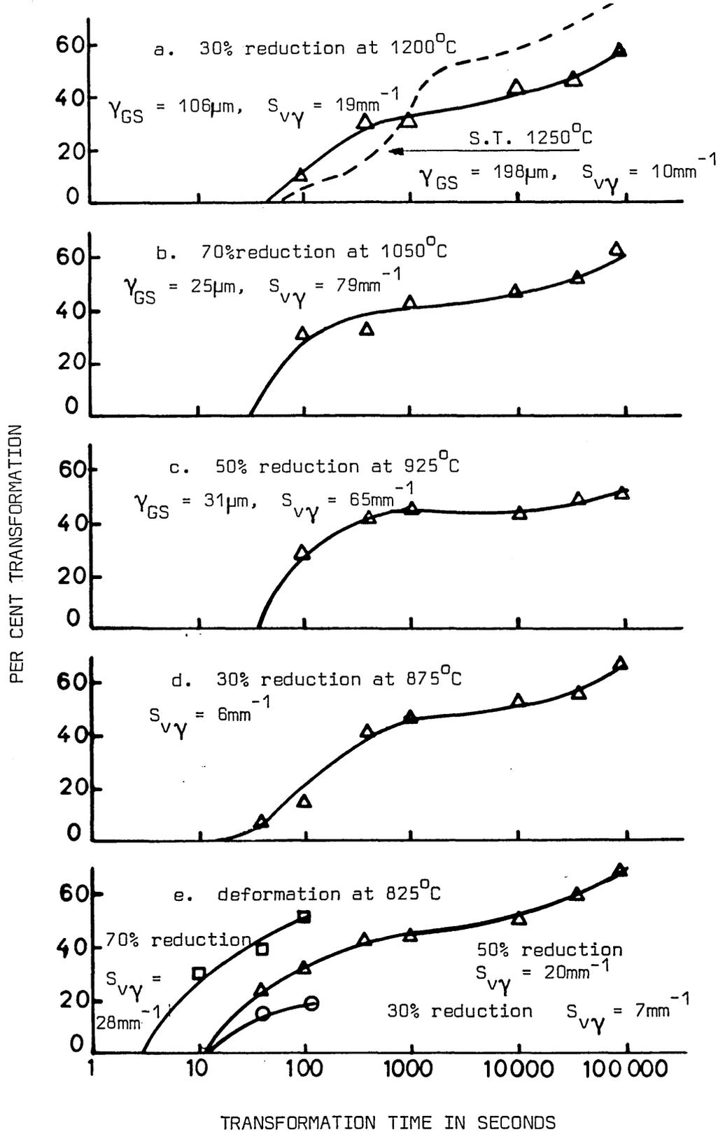
FIG. 101 EFFECT OF DEFORMATION PRIOR TO ISOTHERMAL TRANSFORMATION AT 750°C IN 0.11%C, 1.4/1.5%Mn, 0.13/0.15%V AND 0.004/0.005%N STEEL
