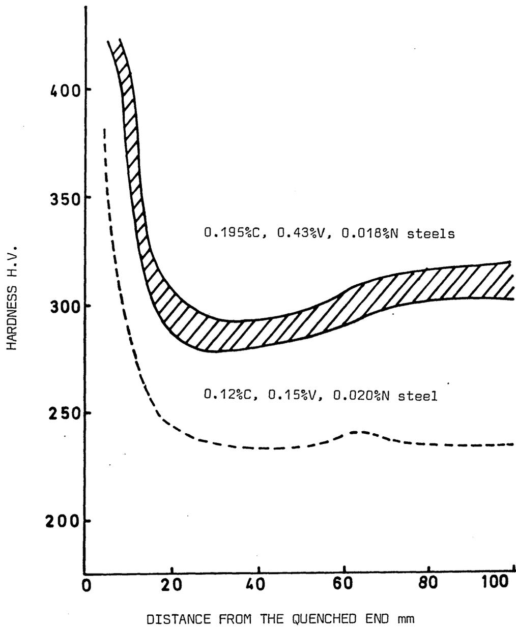
FIG. 73 EFFECT OF SIMULTANEOUSLY INCREASING CARBON AND VANADIUM CONTENT ON THE MODIFIED JOMINY HARDNESS CURVES AUSTENITISED AT 1250°C
