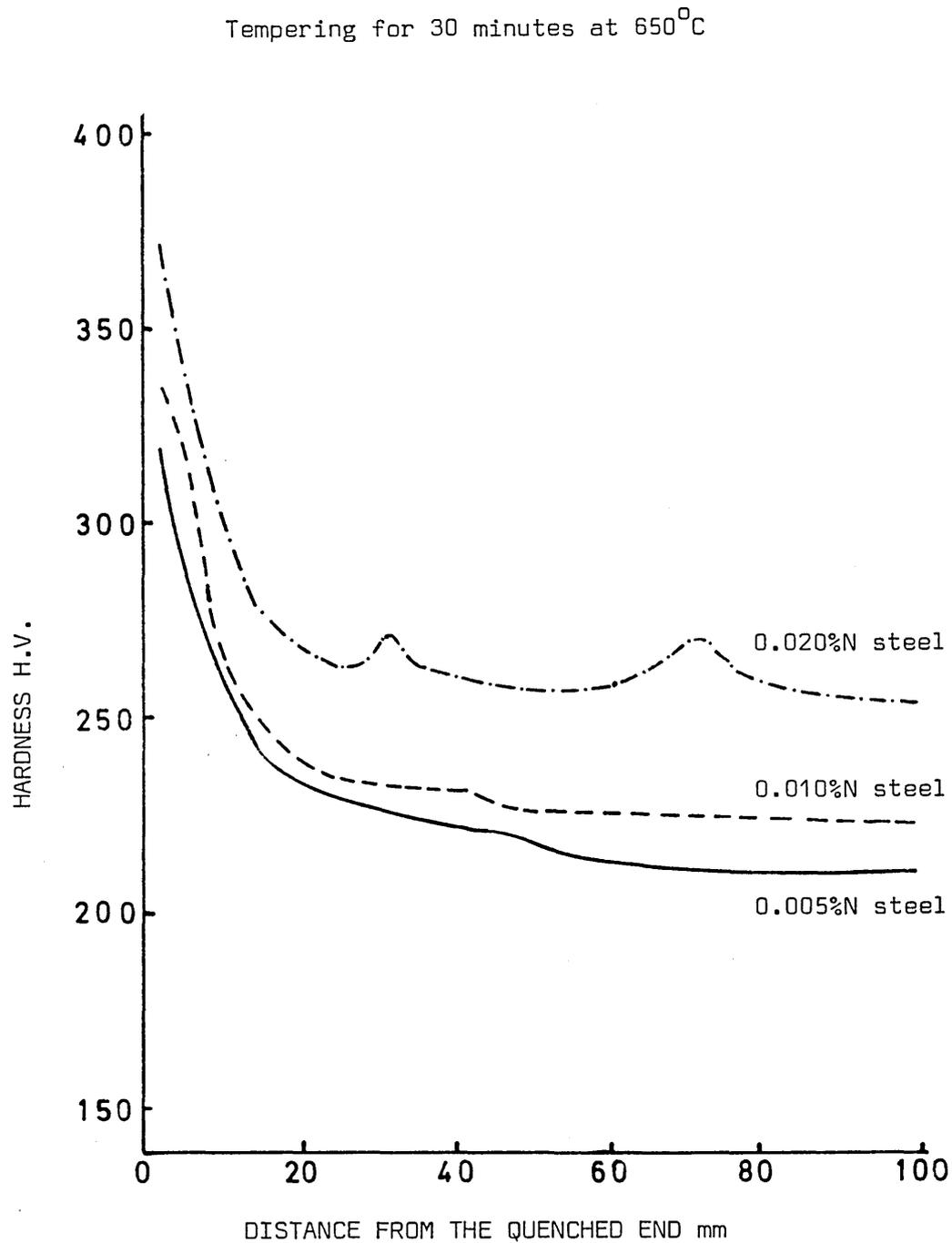
FIG. 80 EFFECT OF INCREASING NITROGEN ON THE TEMPERING OF JOMINY BARS AFTER AUSTENITISING AT 1250°C
