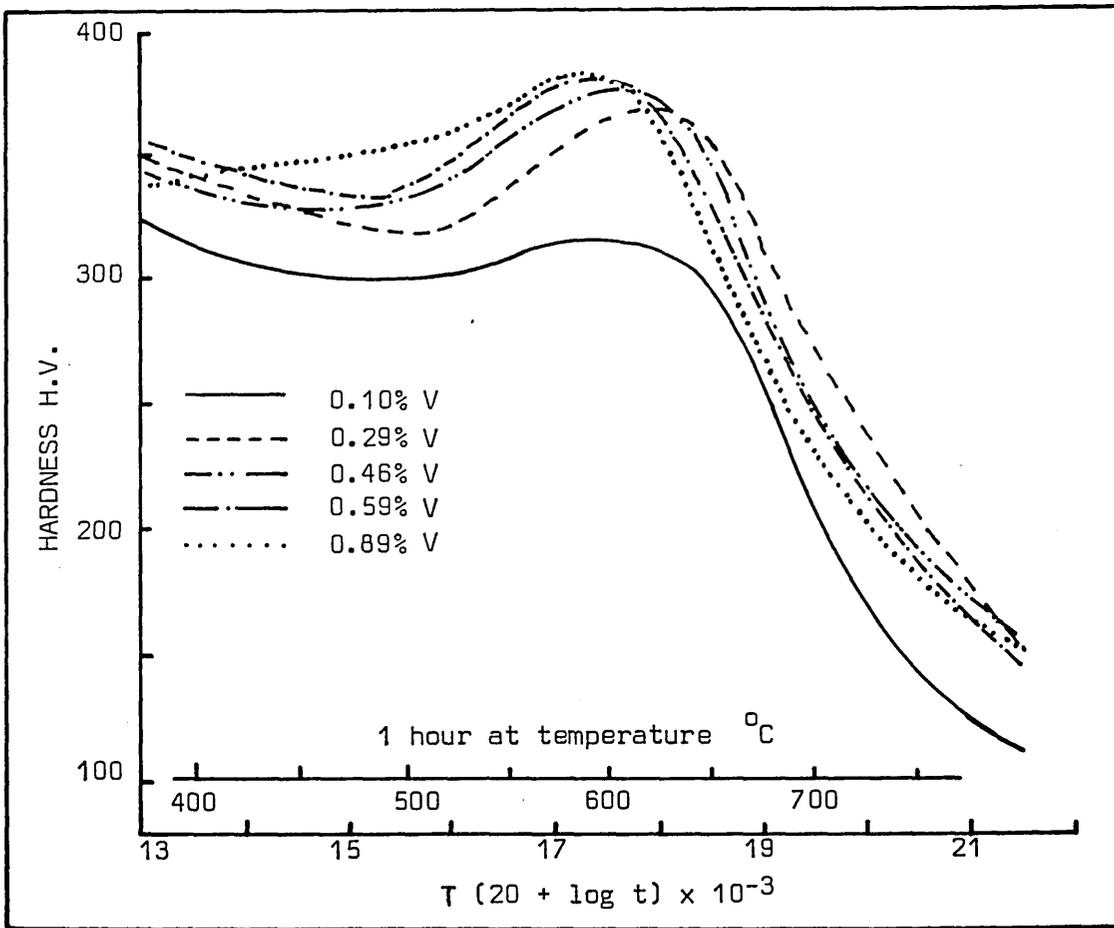
FIG. 30 THE EFFECT OF VANADIUM ON THE TEMPERING CHARACTERISTICS OF WATER QUENCHED STEELS
