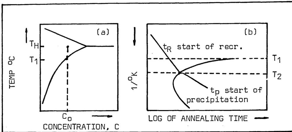
FIG. 13 OCCURRENCE OF RECRYSTALLISATION AND PRECIPITATION
