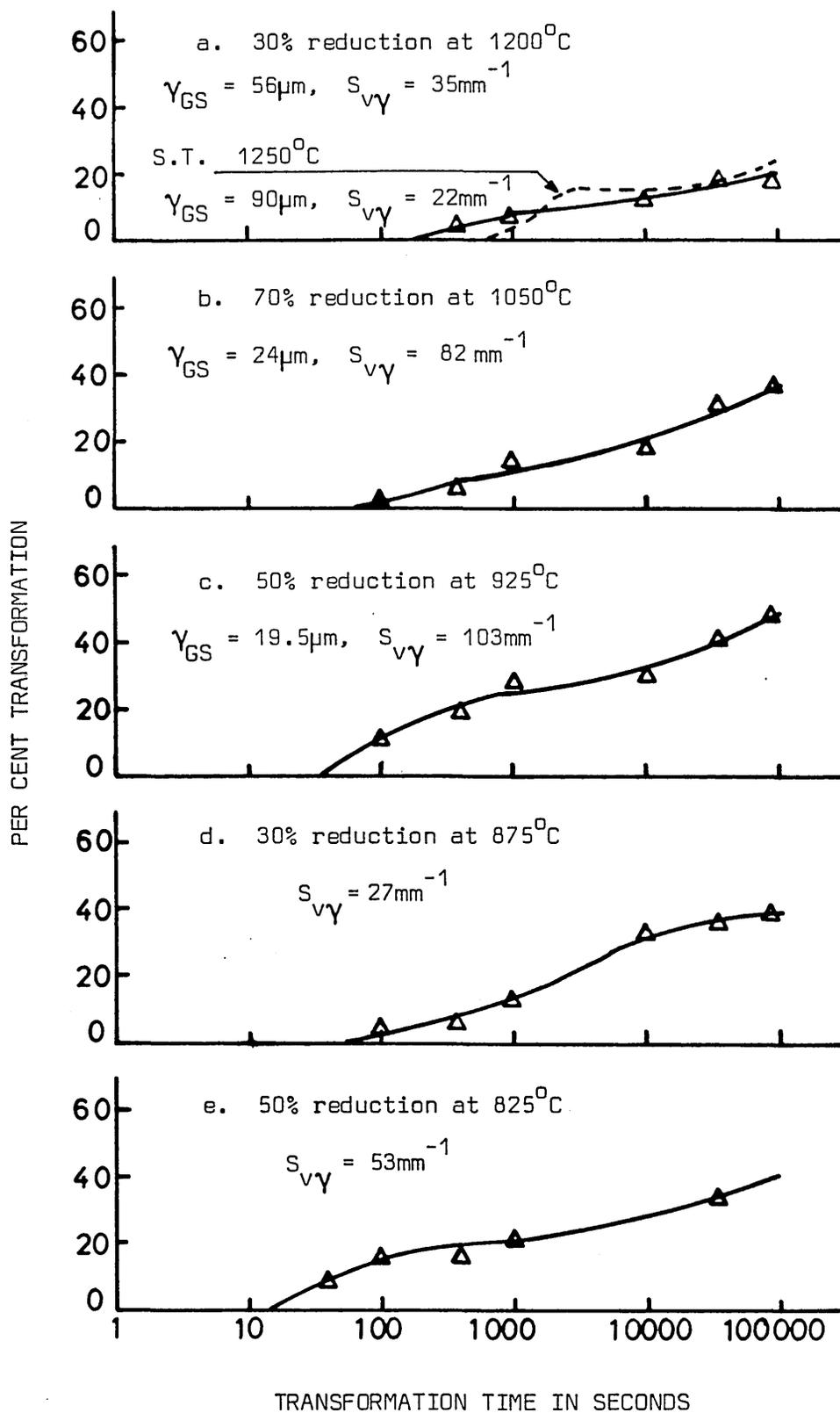
FIG. 102 EFFECT OF DEFORMATION PRIOR TO ISOTHERMAL TRANSFORMATION AT 750°C IN 0.11/0.12%C, 1.6/1.8%Mn, 1.6/1.8%Mn, 0.14/0.15%V AND 0.020/0.021%N STEELS
