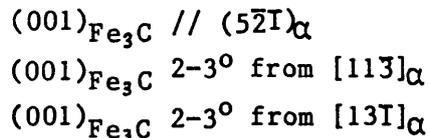
Where there is pro-eutectoid  $\text{Fe}_3\text{C}$  on the austenite grain boundary, it is reported that a different orientation relationship is obeyed because the ferrite will be isolated from the austenite grain into which it does not grow and thus have a simple epitaxial relationship with the cementite, i.e. the Bagaryatski relationship :-
