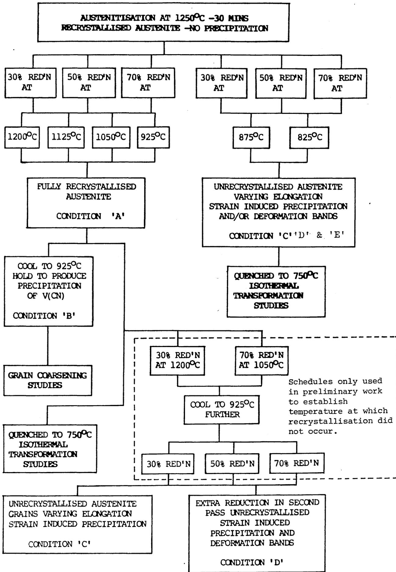
FIG. 32 SCHEMATIC DIAGRAM FOR THE PRODUCTION OF VARYING AUSTENITE STRUCTURES BY THERMO-MECHANICAL TREATMENT
