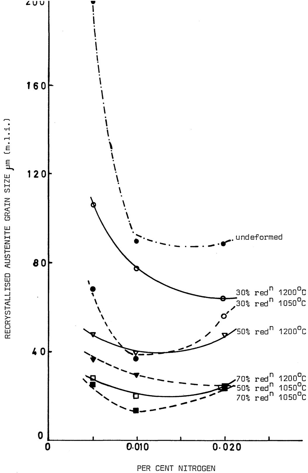
FIG. 86 EFFECT OF NITROGEN ON THE RECRYSTALLISED AUSTENITE GRAIN SIZE IN 0.12% STEELS, FOR DIFFERENT THERMO-MECHANICAL PROCESSING CONDITIONS
