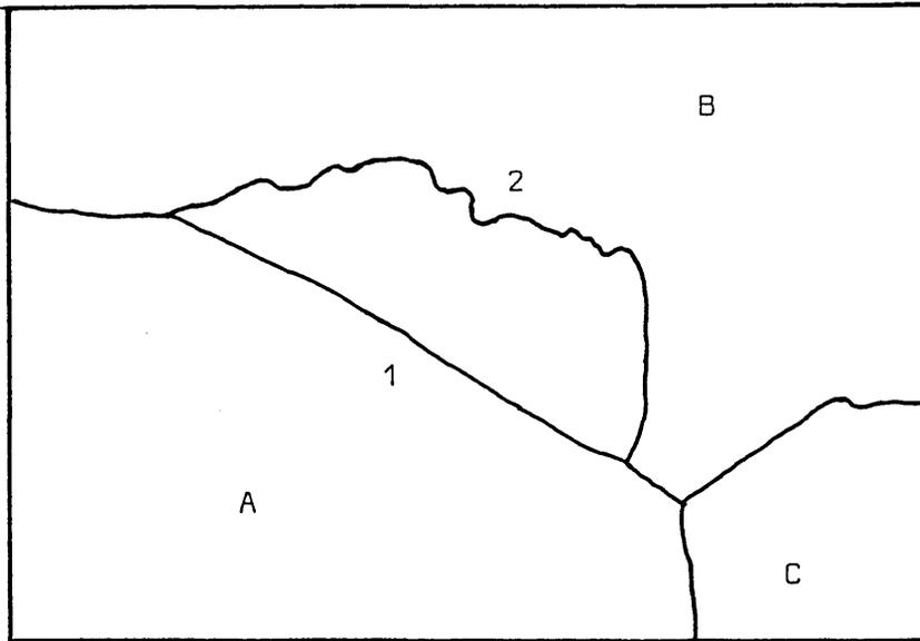
FIG. 5 OUTLINE OF A MICROGRAPH SHOWING STRAIN-INDUCED BOUNDARY MIGRATION IN ALUMINIUM
