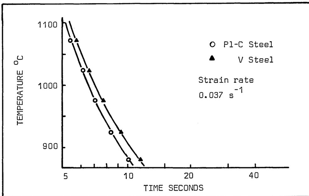
FIG. 21 DYNAMIC RECRYSTALLISATION TIME TEMPERATURE DIAGRAM (RTT)
