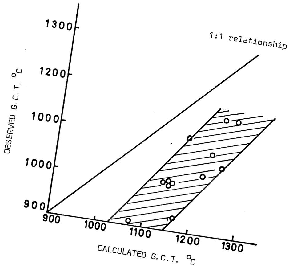
FIG. 109 RELATIONSHIP BETWEEN OBSERVED AND CALCULATED GRAIN COARSENING TEMPERATURE
