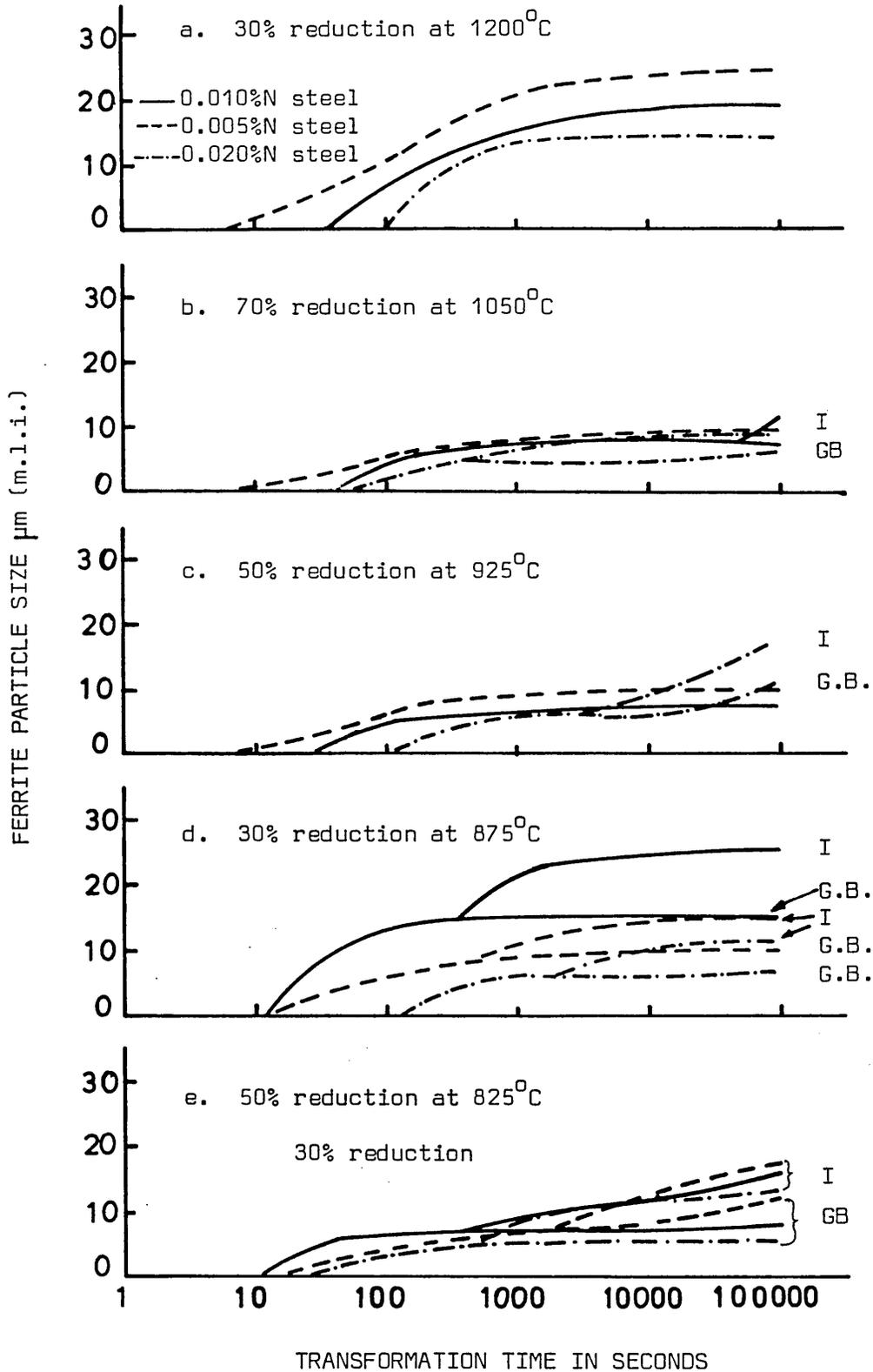
FIG. 107 EFFECT OF INCREASING NITROGEN ON THE FERRITE PARTICLE SIZE SIZE DURING ISOTHERMAL TRANSFORMATION AT 750<sup>o</sup>C IN 0.11/0.0.11/0.128%C, 1.4/1.8%Mn AND 0.13/0.19%V STEELS
