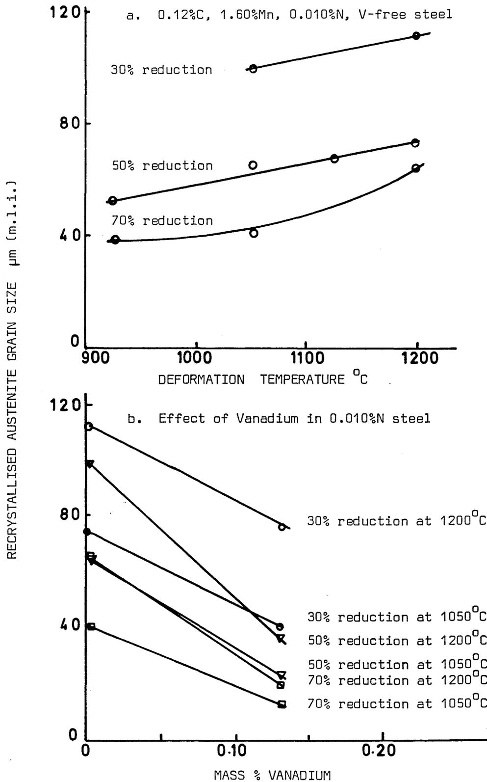
FIG. 83 EFFECT OF VANADIUM ON THE RELATIONSHIP BETWEEN DEFORMATION TEMPERATURE, AMOUNT OF DEFORMATION AND RECRYSTALLISED AUSTENITE GRAIN SIZE.
