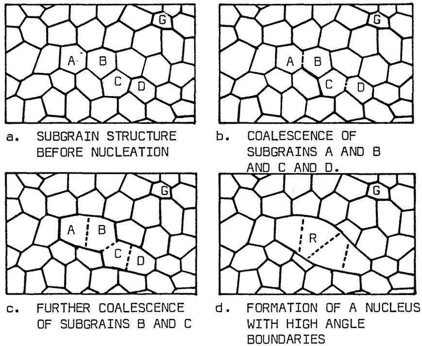
FIG. 4 SCHEMATIC REPRESENTATION OF THE FORMATION OF A PRIMARY RECRYSTALLISATION NUCLEUS BY SUBGRAIN COALESCENCE.
