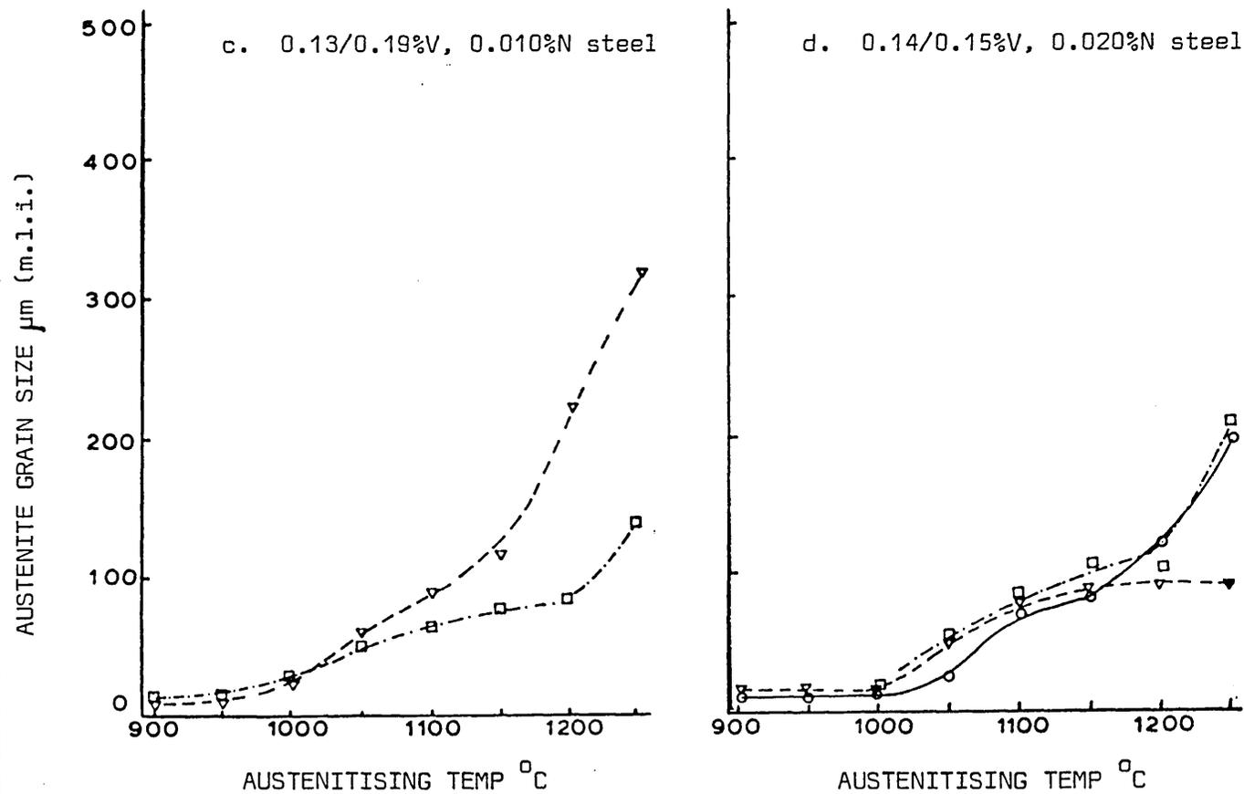
FIG. 49 EFFECT OF CARBON IN 1.6/1.8%Mn STEEL ON THE GRAIN COARSENING CHARACTERISTICS OF AUSTENITE
