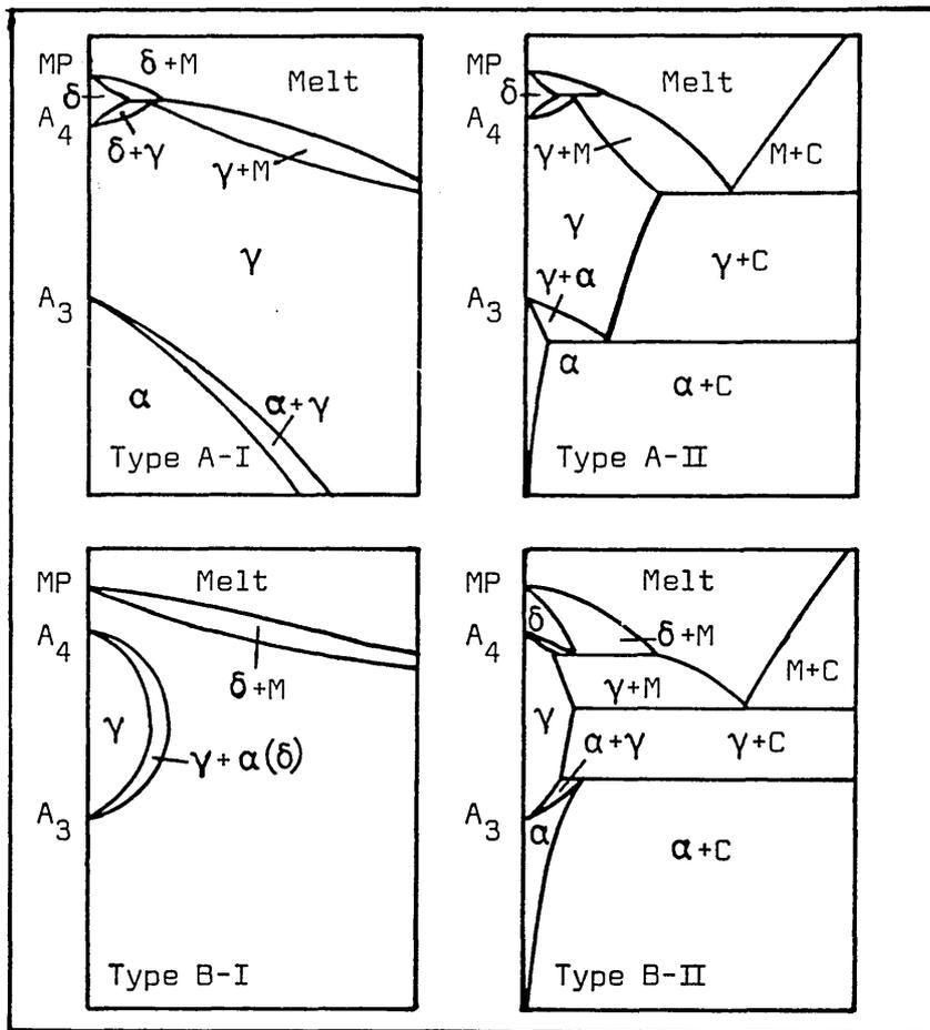
FIG. 25 TWO POSSIBLE TYPES, A AND B, AND THE SUBDIVISIONS I AND II, OF PHASE EQUILIBRIUM DIAGRAMS FOR IRON ALLOYS.
