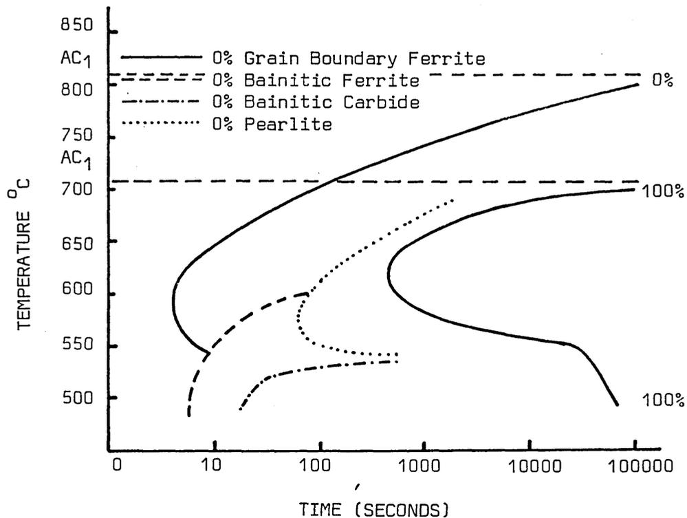
FIG. 67 ISOTHERMAL TRANSFORMATION DIAGRAM FOR 0.12%C, 1.77%Mn, 0.15%V, 0.020%N, STEEL AUSTENITISED AT 1250°C, AUSTENITE GRAIN SIZE 89 μm
