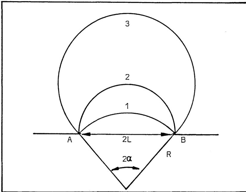
FIG. 7 SCHEMATIC REPRESENTATION OF GRAIN BOUNDARY BULGING.
