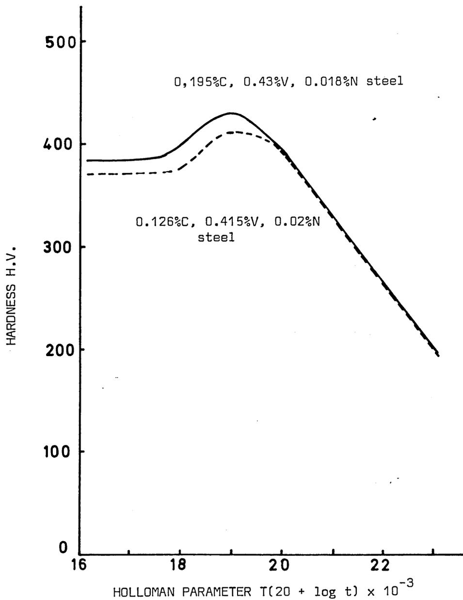
FIG. 59 EFFECT OF CARBON ON TEMPERING CURVE FOR 0.41/0.43%V, 0.018/0.020%N STEEL AUSTENITISING AT 1250°C
