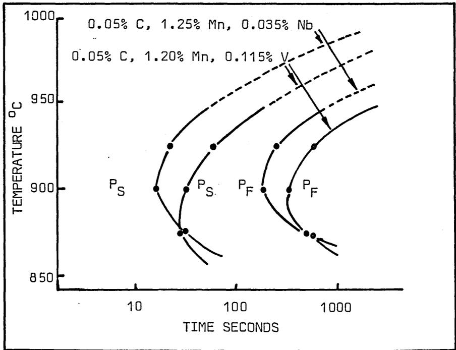
FIG. 20 DYNAMIC PRECIPITATION TIME TEMPERATURE DIAGRAM (PTT)
