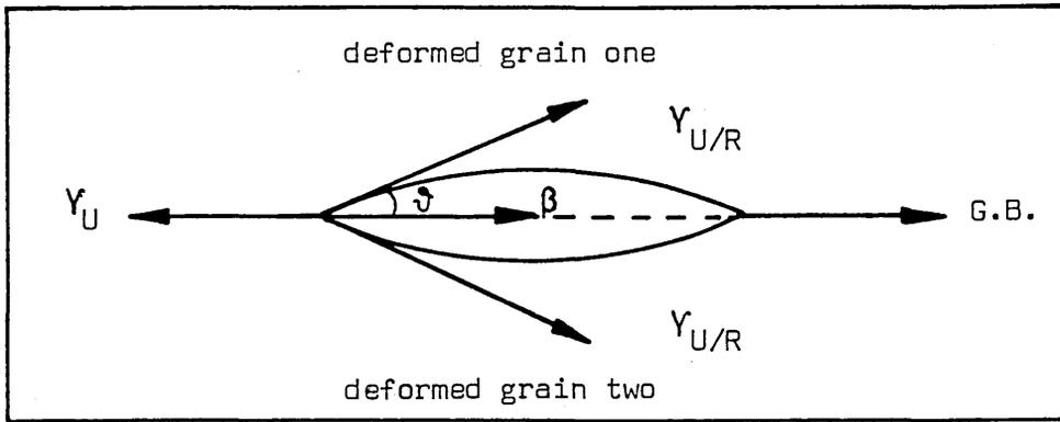
FIG. 1 THE FORMATION OF A  $\beta$  NUCLEUS OF A RECRYSTALLISED STRUCTURE ON THE GRAIN BOUNDARY BETWEEN TWO DEFORMED GRAINS.
