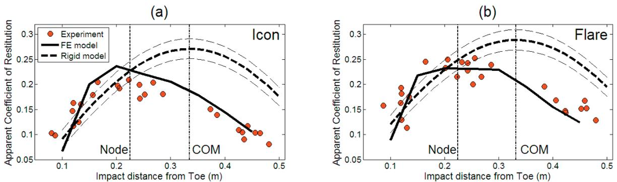
Figure 3 Results for the ball/bat impact a) Icon and b) Flare. Material coefficients for the ball in the FE model were Bat-tuned in Table 2.  $e$  for the rigid body model was  $0.46 \pm 5\%$ . Node corresponds to the Nodal Sweet Spot.
