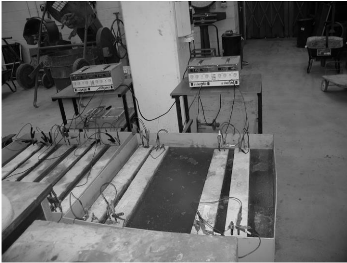
Figure 2. Reinforced concrete beams undergoing accelerated corrosion.
