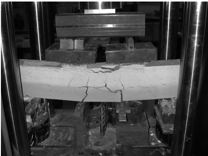
Figure 3. Flexural testing of deteriorated reinforced concrete beams.
