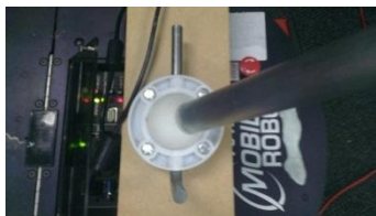
Figure 4, Ball-free mechanism at the base
