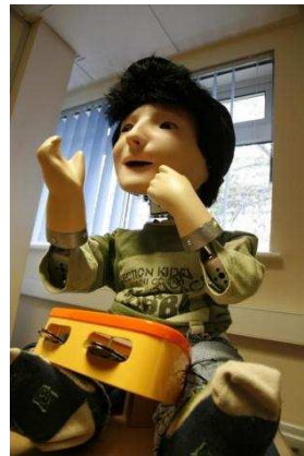
Figure 3, KASPAR robot used to develop robot-assisted therapy applications for children with autism (Courtesy University of Hertfordshire).
