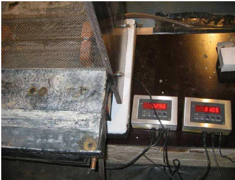
Figure 5 The weighing balance used in the continuation work showing the base with heavy duty gauze so that water discharging through the core can be collected in the trough. (Photograph from Wood, 2010)
