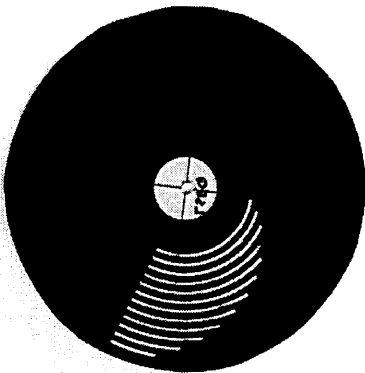
Figure A8.3 Encoder wheel designed to simulate sequential fragmentation and arc ignition initiated at one end of the fuse element
