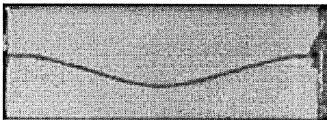
(i) Catenary shaped current carrying 0.2032Ømm/30mm silver wire element with longitudinal disposition below the horizontal origin \approx 6.5 ms after current initiation. ( I_p=320 A)
