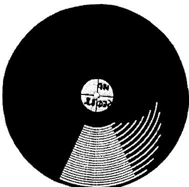
Figure A8.9 Encoder wheel designed to simulate sequential fragmentation and arc ignition and subsequently arc expansion
