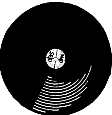
Figure A8.5 Encoder wheel designed to simulate sequential fragmentation and arc ignition initiated in the centre of the fuse element
