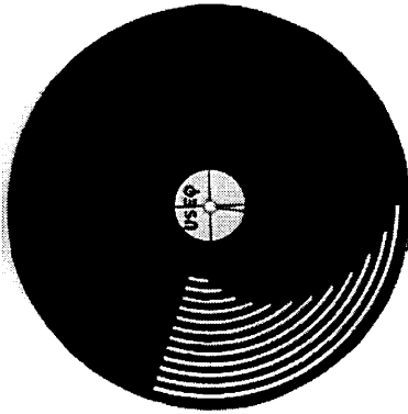
Figure A8.1 Encoder wheel designed to simulate sequential fragmentation and arc ignition initiated at one end of the fuse element
