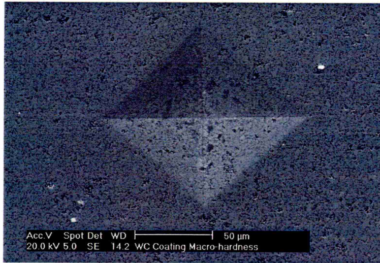
Figure 26: SEM micrograph of a typical 20 kg Vickers indent on a WC-Co tile.
