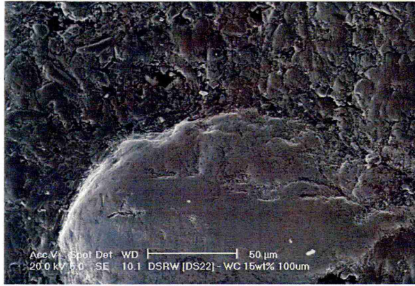
Figure 167: Wear surfaces of (a) 5wt.% 100 µm WC/W 2 C; (b) high magnification; (c) 10wt.% 100 µm WC/W 2 C; (d) high magnification; (e) 15wt.% 100µm WC/W 2 C and (f) high magnification at 130 N applied load, 260 µm silica sand; modified ASTM G65 dry environment.
