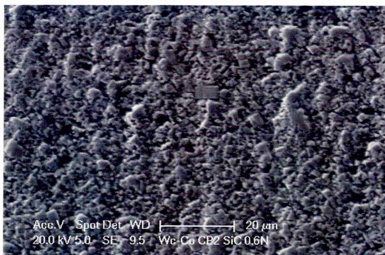
Figure 125: SEM micrograph of MSAW scar on WC-Co tile subjected to wear with SiC abrasive under a load of 0.6 N. The Co binder can be seen to be suffering material loss with the carbides standing proud of the surface.
