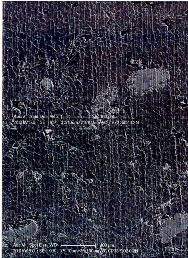
Figure 140: SEM micrographs MSAW scars on mixed ratios of 100 \mu\text{m} WC/W 2 C and 15 \mu\text{m} WC using SiO 2 abrasive over 100 m sliding distance.
