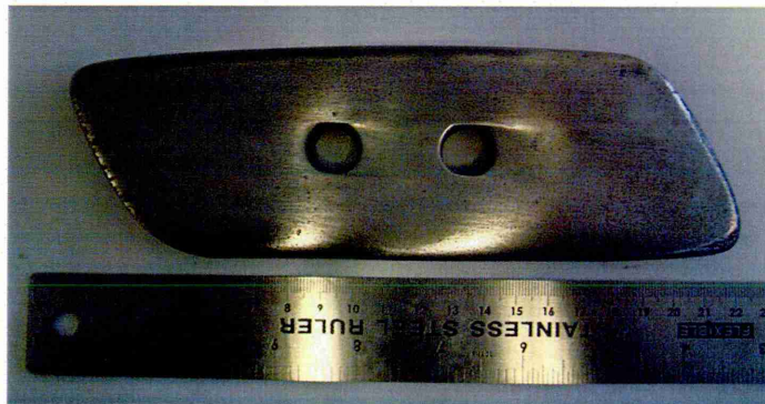
Figure 32: Boron steel reversible point removed from service.
