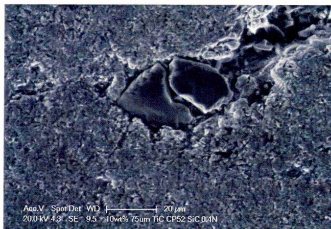
Figure 124: SEM micrograph of MSAW test scar on 10wt.% 75 \mu\text{m} TiC produced using SiC abrasive at a load of 0.4 N over a sliding distance of 50 m. A TiC particle is visible which has not bonded with the matrix material and has suffered brittle fracture in the process of wear.
