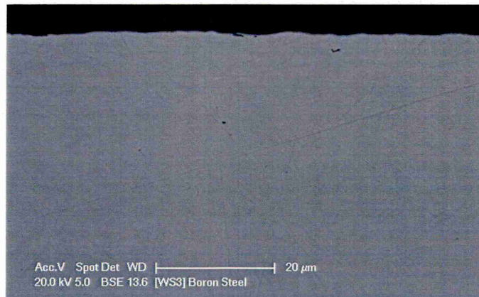
Figure 174: Cross-section of WSRW scar on boron steel 90 degrees to the rolling direction.
