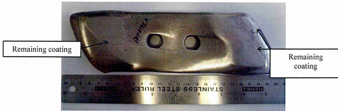
Figure 35: Armatech coated boron steel reversible point soil wear.
