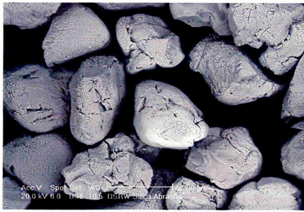
Figure 50: SEM micrograph of 260 µm silica sand used in ASTM G65 tests.
