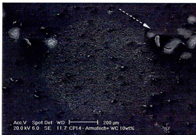
Figure 134: Typical wear scar from MSAW testing using \text{SiO}_2 over 100 m sliding distance on \text{WC/W}_2\text{C}(10)_{100\text{J}} . Arrow denotes direction of ball rotation.
