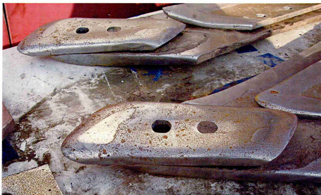
Figure 186: Photographs of ploughshares following 110 acres of testing, some patches of coating material can be still seen.
