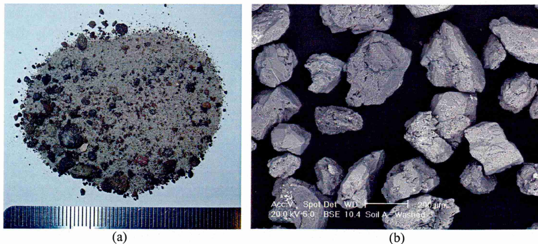
Figure 53: Photograph of dried soil and SEM Micrograph of silica particles.
