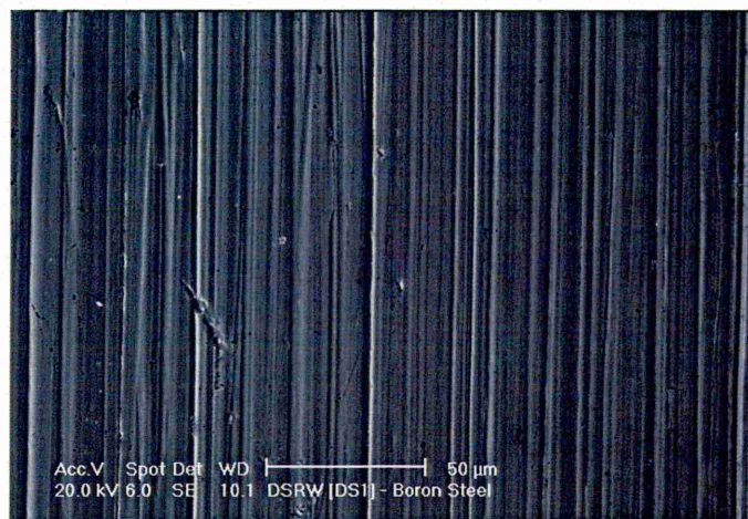
Figure 161: Wear surfaces of boron steel at 130 N applied load, 260 \mu\text{m} silica sand; modified ASTM G65 dry environment.
