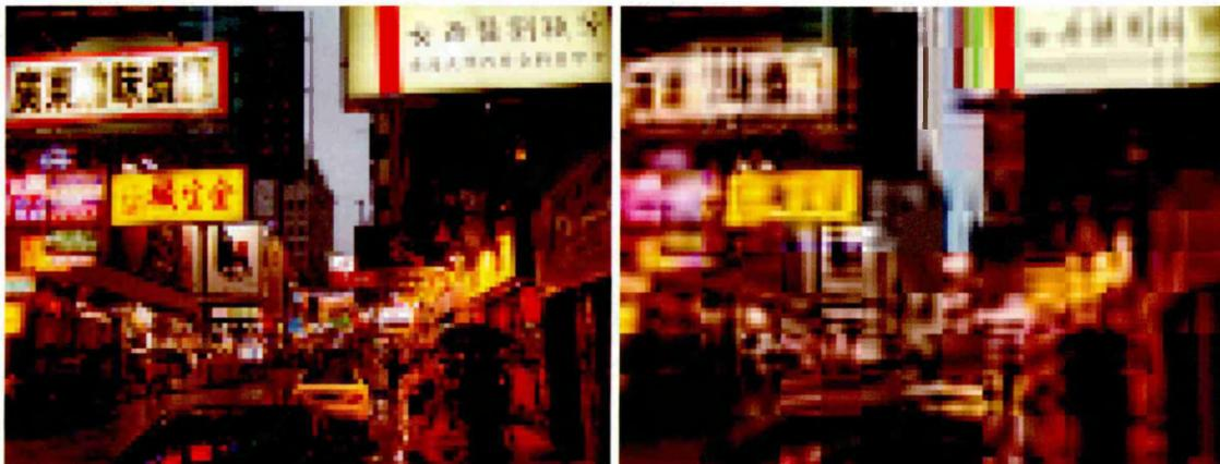
Figure 4.8: Low resolution colour image using lossless **PNG** and (extremely) lossy **JPEG** compression
