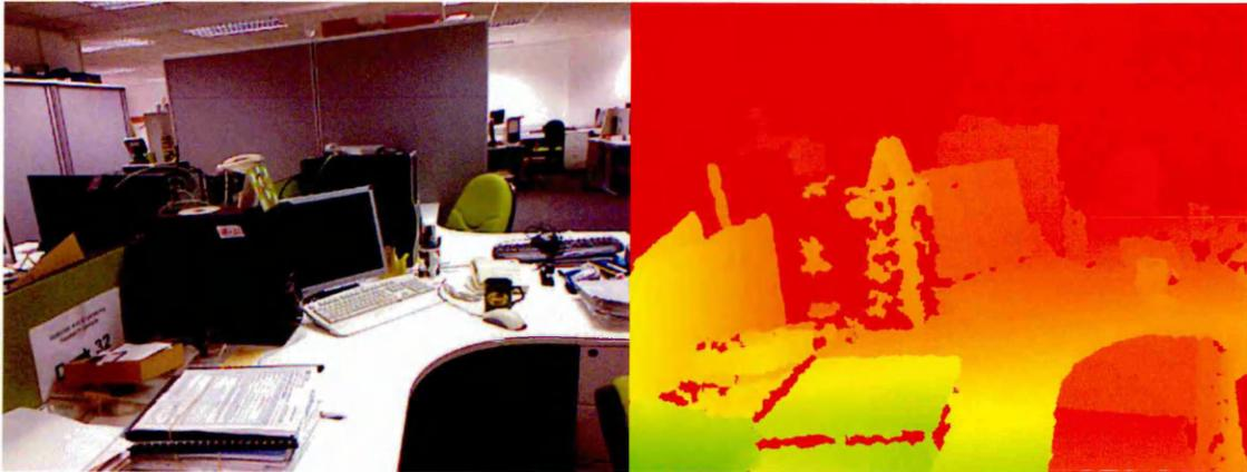
Figure 4.15: RGB- and depth-image acquired with an **RGBD** sensor
