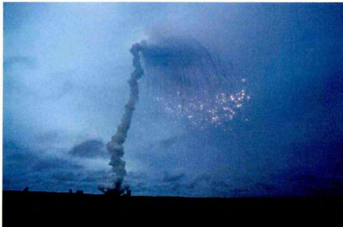
Figure 1.7: Ariane 5 disaster caused by numerical overflow
