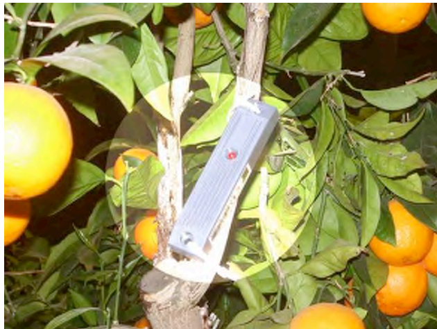
Fig. 1 The long-range RFID tag placed on a fruit tree.
