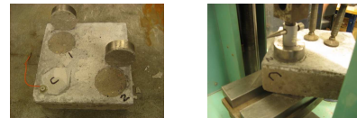
Figure 3 Photographs Showing Pull-off Bond Tests
