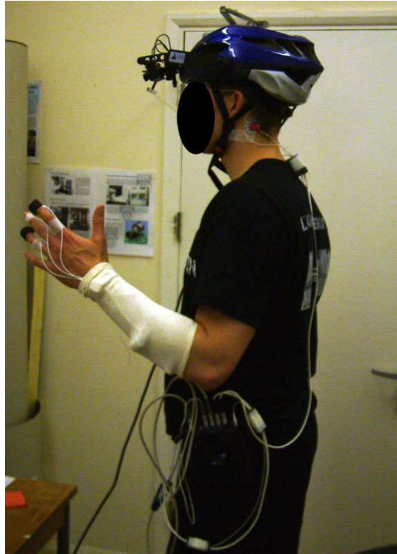
Figure 7: Wireless psychophysiological monitoring setup incorporating GSR, Skin Conductance and Eye Tracking facilities
