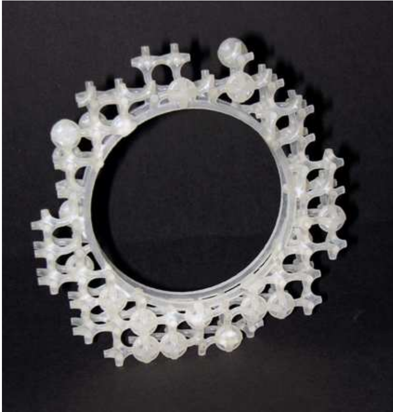
Figure 12: Bangle form created using Invision 3D printer
