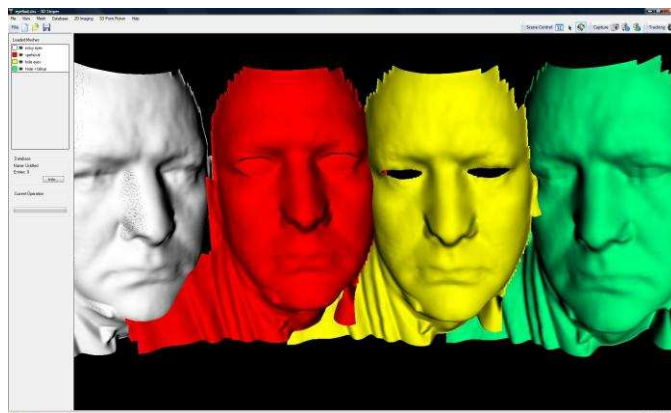
Figure 5: Comparative analysis of noise removal around the eyes. The white model shows the original mesh; red: fitting an elliptical mask around the eyes and filling with a spherical surface centered at 40mm behind the model; yellow: punching an elliptical hole around the eyes; green: filling the elliptical hole with bilinear interpolation.
