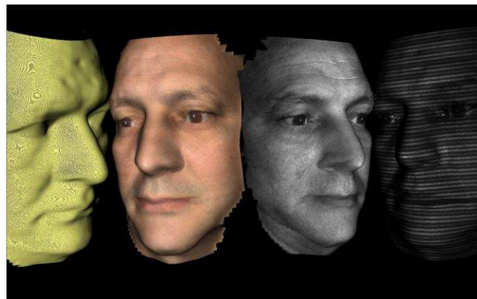
Figure 6. Triangulated mesh (left), with color and black and white texture mapping (centre) and with original stripe pattern (right)
