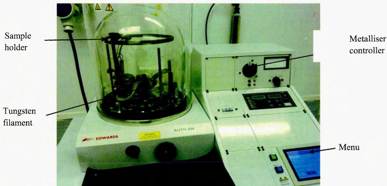
**Figure 3.1:** A photograph of an EDWARD metalliser.
