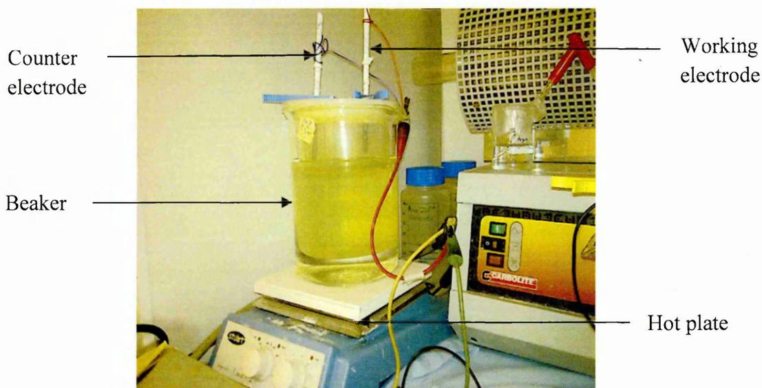
**Figure 2.10 (b):** A photograph of a typical two electrode set-up.
