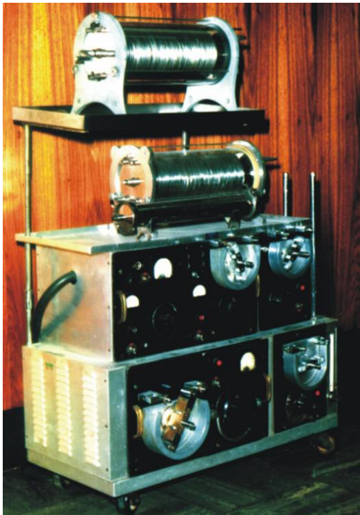
Fig. 4. The first extra-corporeal circulation machine, in 1958.
