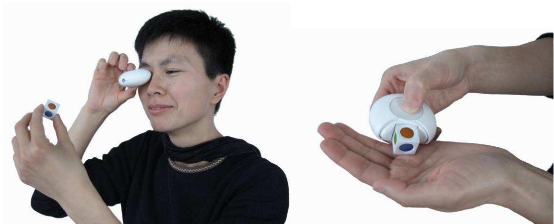
Fig. 2-3: Usage of the mobile EPR device
