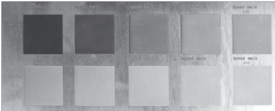
Figure 14 Shikudo (2%Au) alloy laser marked using square raster patterns. The laser speed for each square was, left to right top row, 50 to 500mm/s steps of 50mm/s.
