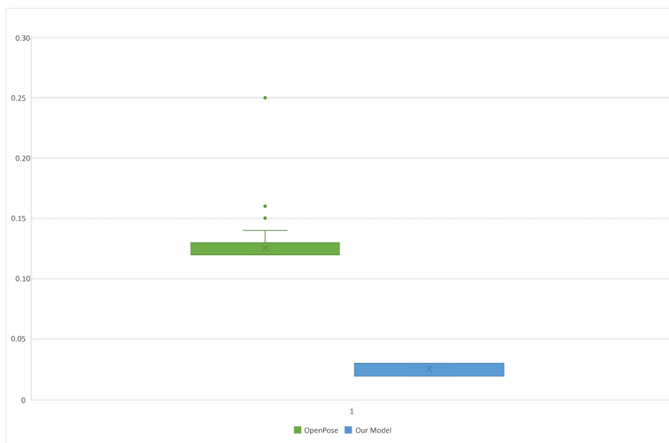
Fig. 6 Computational performance in seconds of the OpenPose algorithm and our model on NVIDIA Jetson TX2
