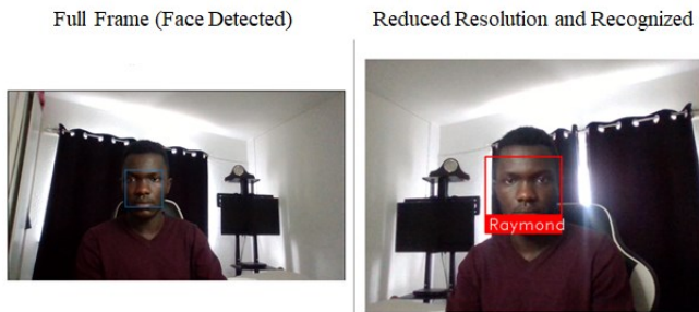
Figure 1: Face Detection and Recognition
