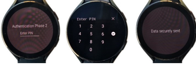
Figure 7: Smartwatch Authentication Initiation from the user
