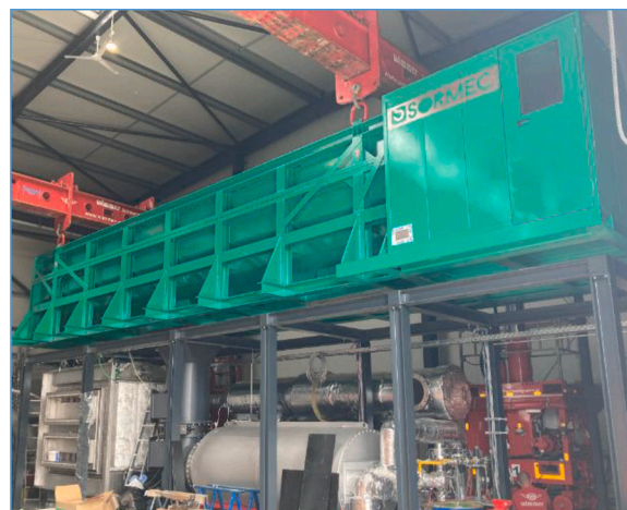
Fig. 8. Auger reactor, combustion chamber, and post-reformer of the TCR-500 plant.
