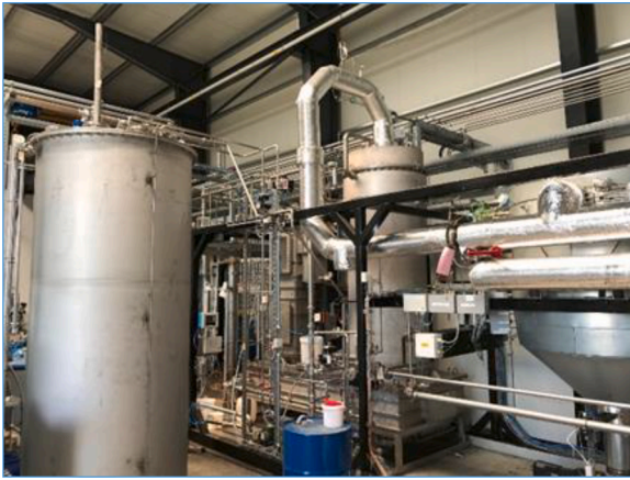
Fig. 9. Hot gas filter and condensation stage of the product gas train of the TCR-500 plant.
