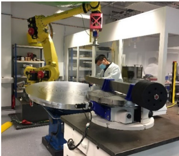
Fig. 14 Swing-arm profilometer integrated into the polishing cell
