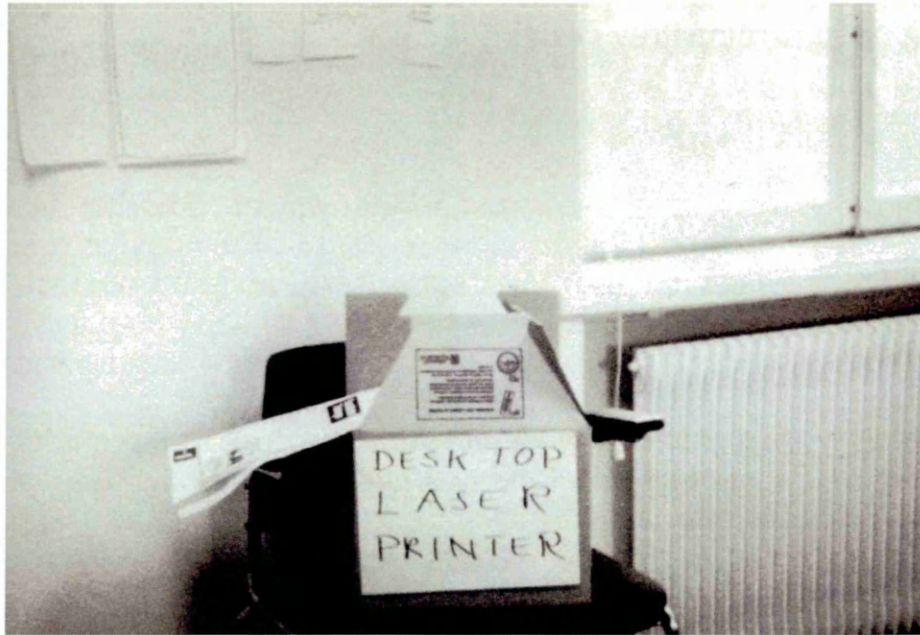
Figure 3.2 a low fidelity mock-up of a laser printer (image courtesy of Pelle Ehn)
