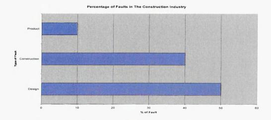
**Figure 3.3:** Percentage of Failures / Faults in the Construction Industry (After Building Research Establishment, 1982)
