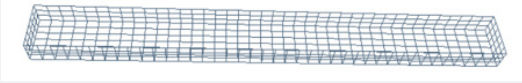
Figure 3: Total 516 panels are used with 3 panel in vertical direction, 6 panels in transverse direction and 40 panels in longitudinal direction.
