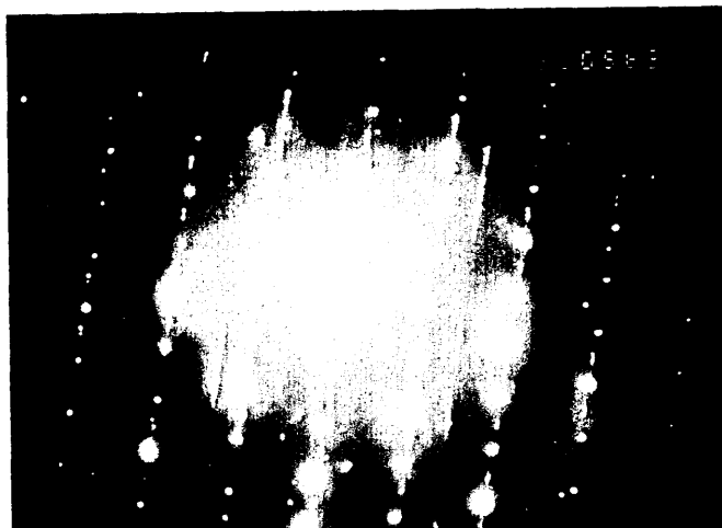
Figure 15 Electron Diffraction Pattern from Intragranular Carbides shown in figure 14 - crystal structure determined as M_7C_3
