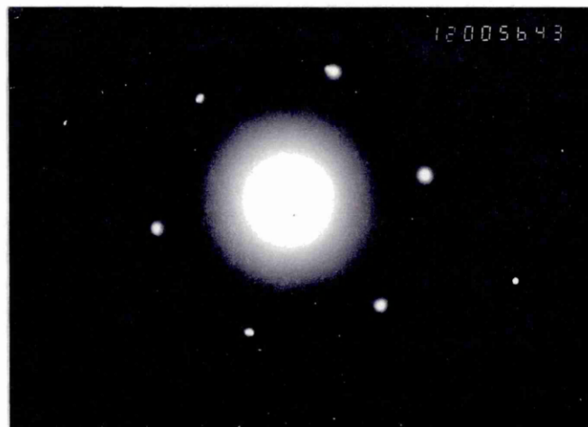
Figure 19 Electron diffraction pattern from smaller intragranular Carbides shown in figure 18 - structure determined as Titanium Carbide (TiC)
