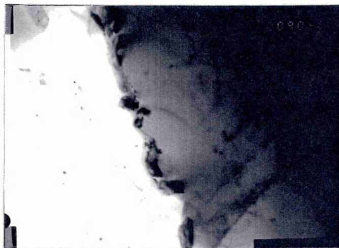
a) Alloy 1B, aged 650°C 16 hours. Growth of discrete grain boundary carbides.
