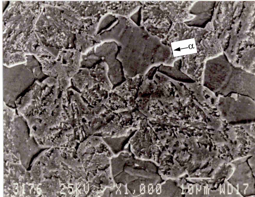
Figure 4.11 SEM micrograph showing the microstructure consisted of upper bainite and considerable volume fraction of ferrite, austenitised at 950°C for 20 mins and then cooled at 0.3°C/min
