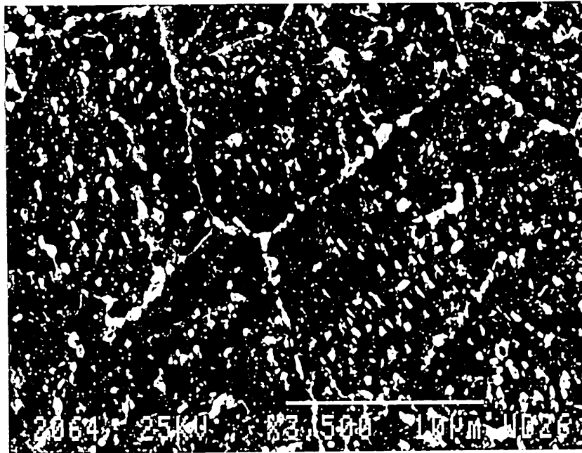
Figure 5.9 Austenitised at 975°C for 5 hrs followed by furnace cooling and then tempered at 700°C for 100 hrs
