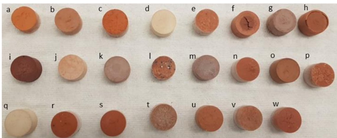
Figure 3. Optical image of ceramic samples showing a representative heavy clay ceramic sample (a) and those produced by incorporating 23 different types of waste ashes into the heavy clay at 20wt% (b-w).
