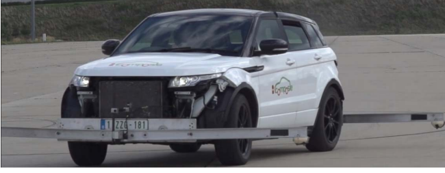
Fig. 13. iCOMPOSE electric vehicle demonstrator with the Corrsys Datron sensor mounted at the front end.
