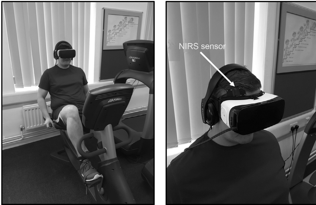
Fig. 1. Equipment setup for the high immersion (HI) condition. NIRS = near-infrared spectroscopy.
