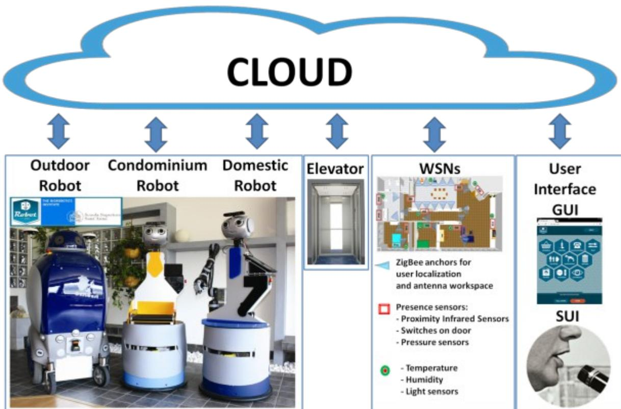
Figure 1 Robot-Era architecture
