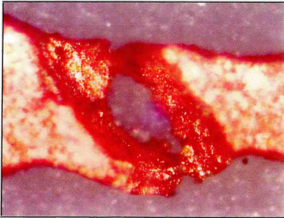
Figure 5-60. Crater. Planar view. Sample E-6, notch D-1. Mag. 330x.
