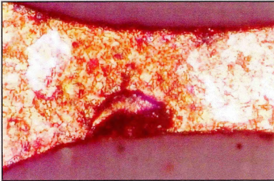
Figure 5-56. Small cavity. Planar view. Sample E-1, notch D-2. Mag. 640x.
