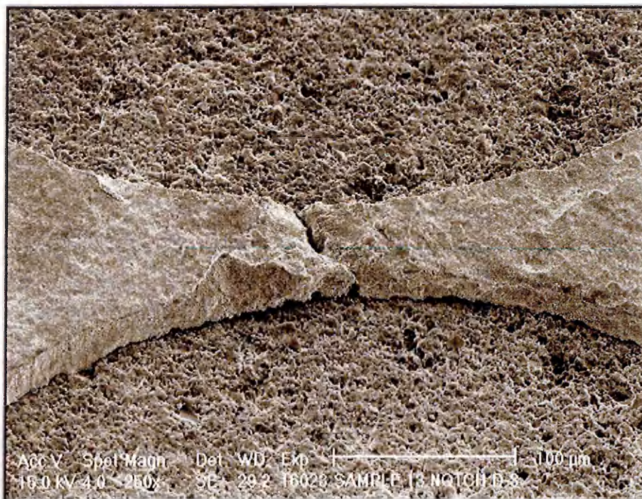
Figure 5-45. Crack propagation – long crack. Sample E-6, notch D-3. Mag. 330x.
