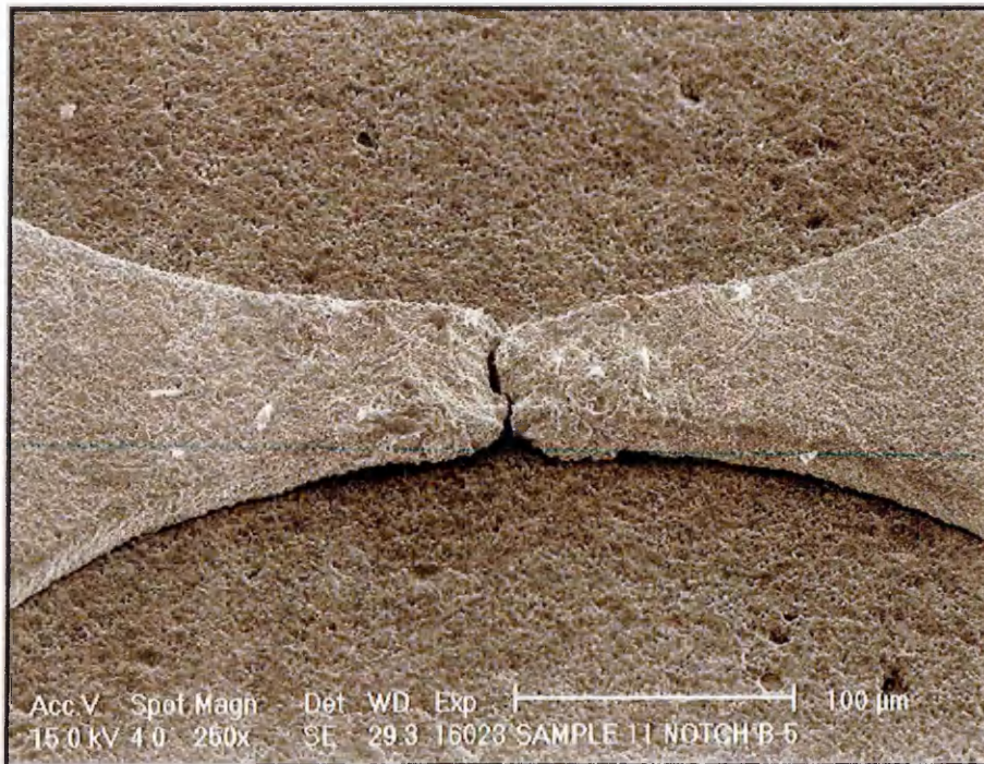
Figure 5-47. Crack propagation – long crack. Sample E-5, notch B-5. Mag. 330x.
