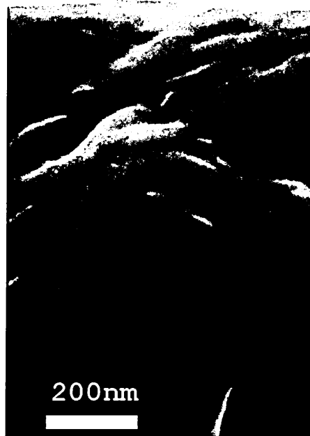
Figure 4.22: Cross-section of a corner of a via coated by 4000 W ICIS at a pressure of 13 Pa
