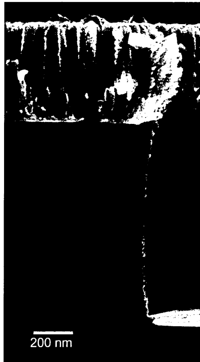
Figure 4.39: Close-up of the corner of the via from figure 4.37 (6.4 Pa). Dendritic growth of the Ni coating can be seen along with the perpendicular growth on the sidewalls.
