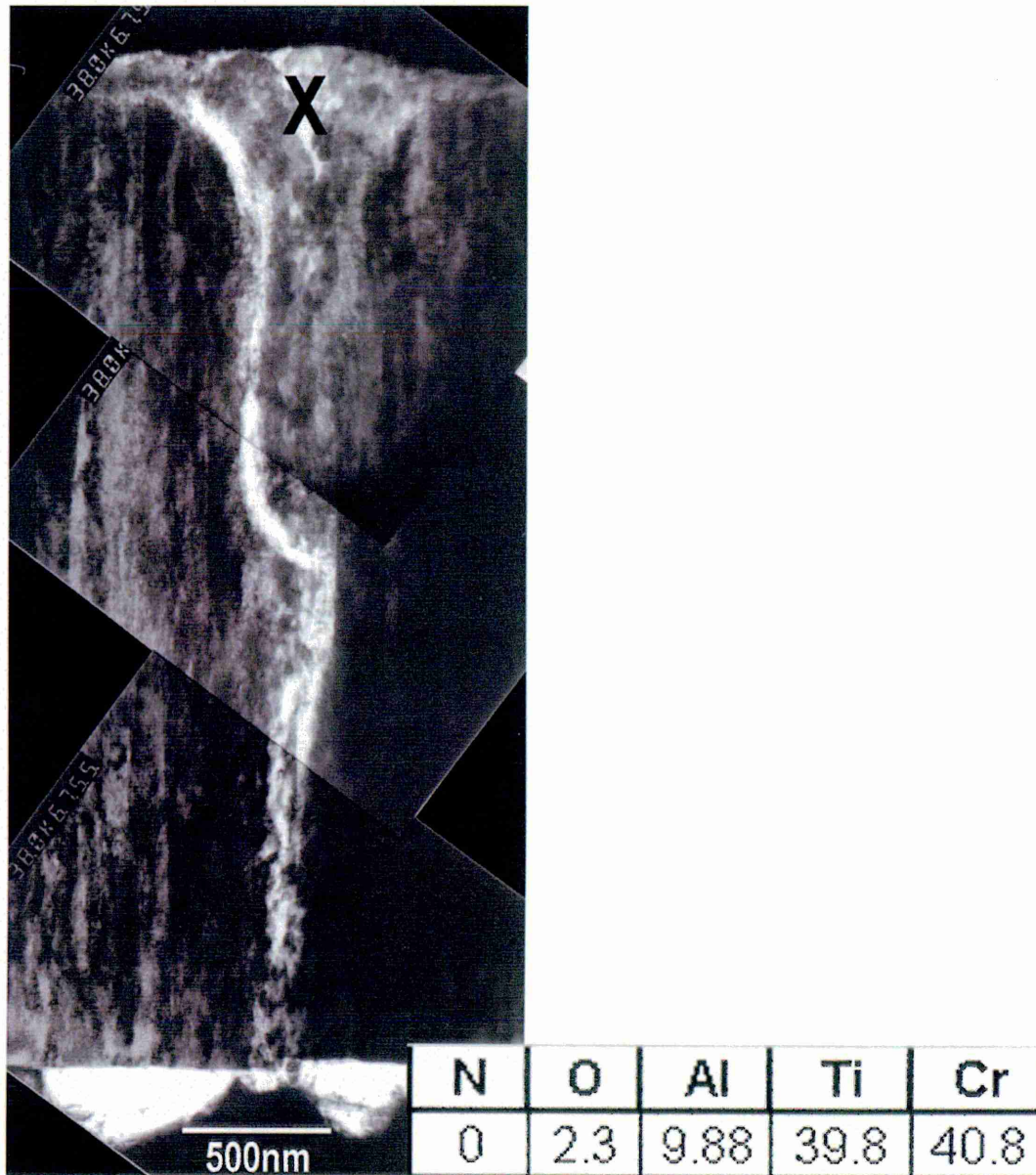
Figure 4-18: TEM BF micrograph with EDX spot analysis on TiAlN/CrN after heat treatment for 1h at 900°C
