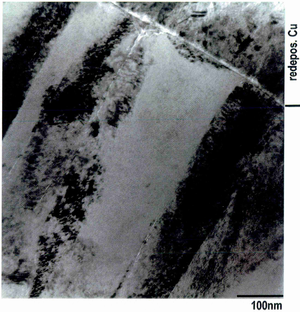
Figure 8-3: TEM BF image of the coating surface of the as-deposited TiAlN/CrN coating
