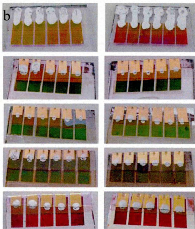
Figure 7.1 (a) Schematic diagram of cross section for top illuminated inverted OSC devices on metal substrates, (b) photos of a pair of real devices on ITO-coated glasses, SS, Cr-Al, Ti-S, and pure Al, from top to bottom. (Note: not to scale).
