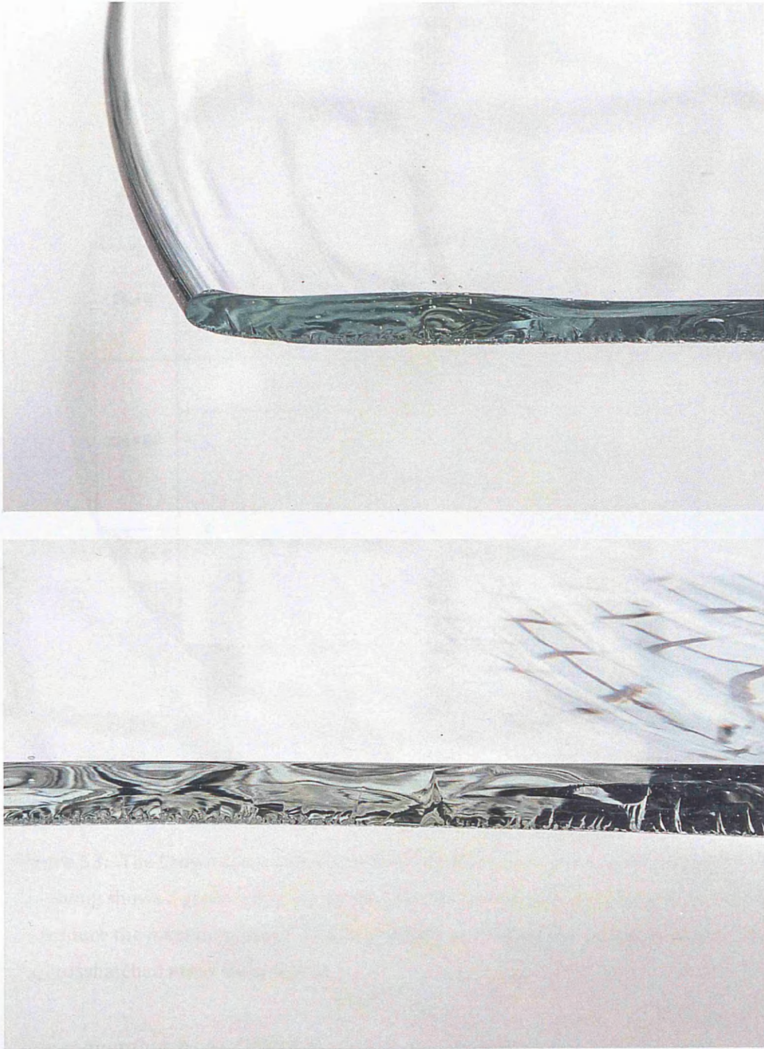
Figure 52: Crown Glass cross section (edge and centre of the disks' cross-section). Photographs: Marcus Sarko, (2015)
