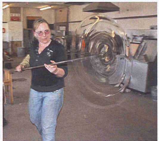
Fig 4. Diderot and d'Alembert's Encyclopedia Fig 5. Ingrid Phillips demonstrating the (1751) Crown Glass, Plate 16. Crown Glass method at the glass department of Edinburgh College of Art (May 2010). Photograph: Jerome Harrington
